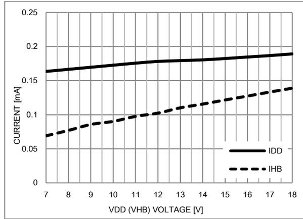
Figure 6. Quiescent Current vs.  $V_{DD}$  ( $V_{HB}$ )
