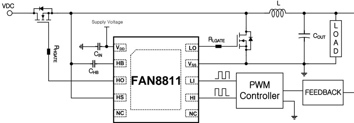
Figure 1. Application Schematic – Synchronous Buck Converter
