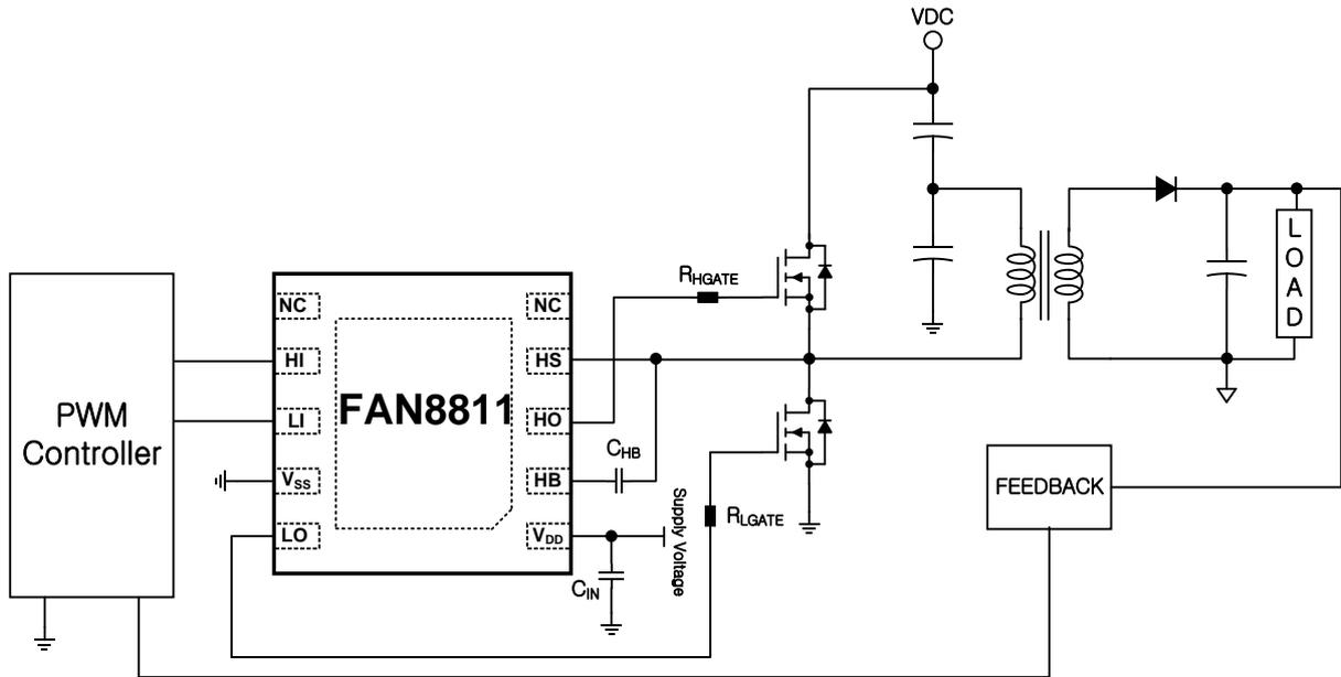
Figure 2. Application Schematic – Half Bridge Converter
