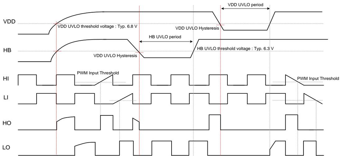
**Figure 24. Overall Operation Timing Diagram**
