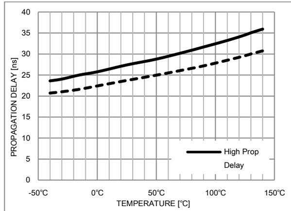
Figure 18. High Side Propagation Delay vs. Temperature
