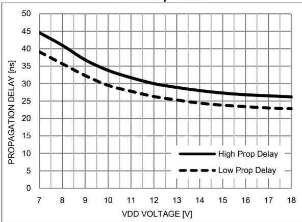
Figure 19. Low Side Propagation Delay vs.  $V_{DD}$
