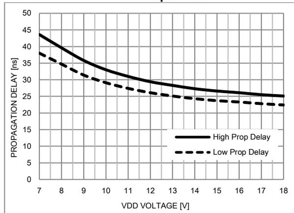
Figure 20. High Side Propagation Delay vs.  $V_{HB}$
