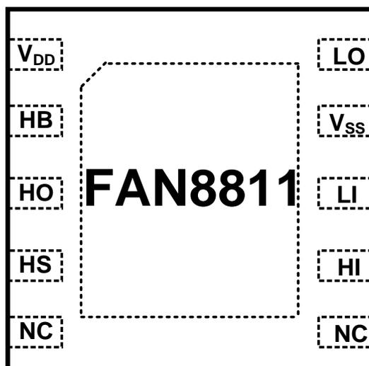
Figure 4. Pin Assignments – 10 Lead MLP (Top View)
