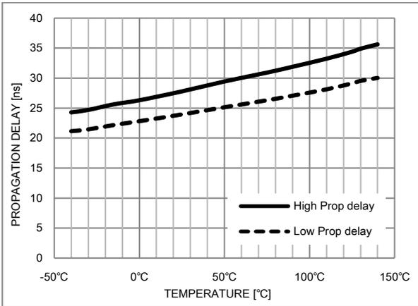
Figure 17. Low Side Propagation Delay vs. Temperature
