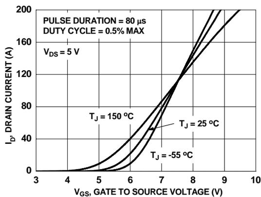
Figure 5. Transfer Characteristics
