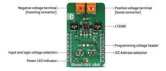
As already mentioned, the LTC3582 features a set of programmable parameters, which can be accessed via the I2C interface. These parameters include configuring the output voltages, power sequencing, and output voltage ramp rates. An onboard OTP non-volatile memory can be programmed with values that will be used at the startup. The command register (CMDR) is reset to 0x00h upon powering up, which disables the
