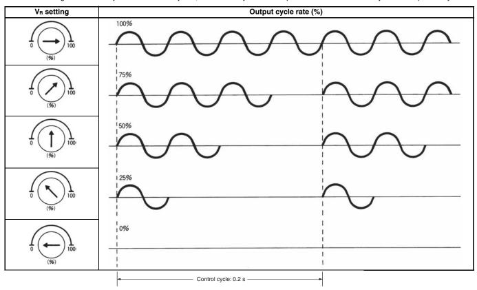
Note: The resistance is 50 k $\Omega$  at 100% and 0  $\Omega$  at 0%.
