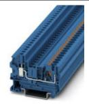
Feed-through terminal block, Connection type: Push-in connection, Screw connection, Cross section: 0.2 mm<sup>2</sup> - 6 mm<sup>2</sup>, AWG :24- 12, Width: 6.2 mm, Color: blue, Mounting: NS 35/7,5, NS 35/15
