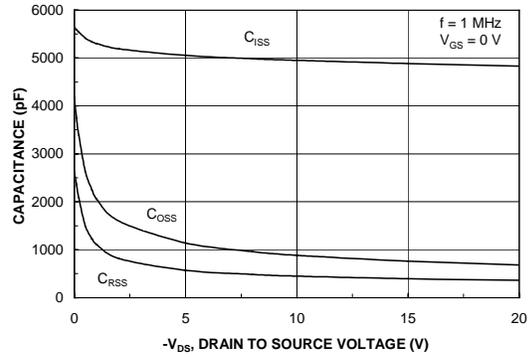
Figure 8. Capacitance Characteristics.
