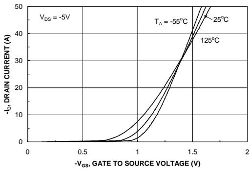
Figure 5. Transfer Characteristics.
