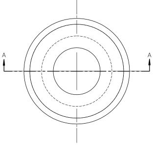
For use with panels of: Max Thickness = 0.063" Hole Dia. = 0.375"
