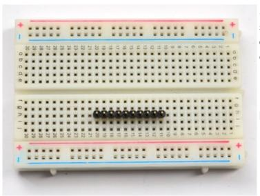
Sometimes we toss in a longer strip, but its easy to break it down, just use pliers or diagonal cutters to snap it down to 10 pins.
