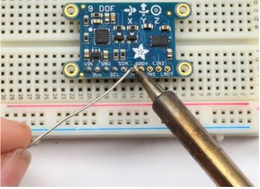
Heat up your soldering iron and once it is ready, solder all 10 pads to the header, making sure to check that there is plenty of solder to make a mechanically strong connection and there's no solder bridging either.
