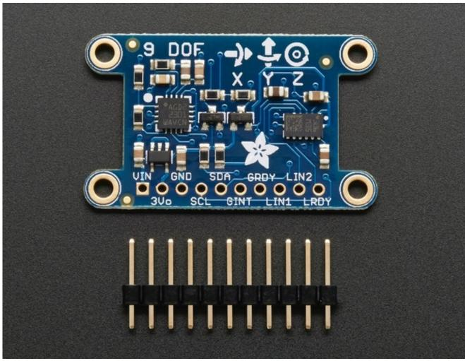
All of the sensors on the Adafruit 9DOF breakout communicate via a two-pin I2C bus, making it relatively easy to setup with a minimum number of cables:
