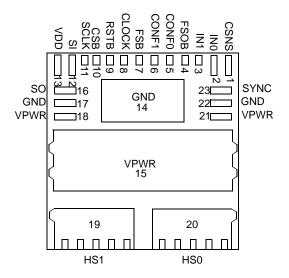
Figure 3. 10XS4200 Pin Assignments
