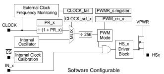
Figure 12. Internal and External Clock Operation
