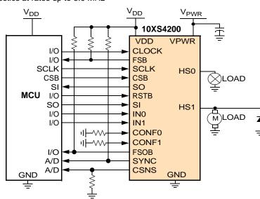
Figure 1. Simplified Application Diagram
