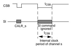
When the duration of the negative CSB pulse is outside a predefined time slot (from  $t_{CSB(MIN)}$  to  $t_{CSB(MAX)}$ ), the calibration event will be ignored and the internal clock frequency will remain unchanged. If the value ( $f_{PWM(0)}$ ) has not been previously calibrated, it will remain at its default level.
