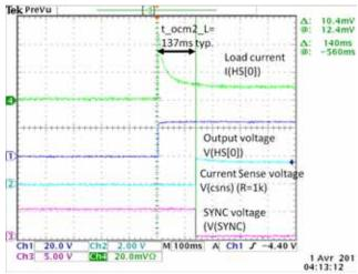
Figure 13. Current Sense Blanking During Over-current Window Activity
