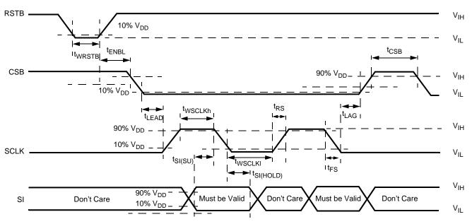
Figure 7. Timing Requirements During SPI Communication
