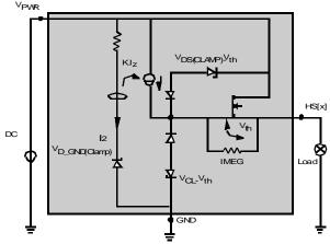
Figure 15. Supply and Output Voltage Protections
