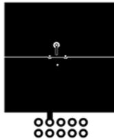
a.  $65^\circ\text{C}/\text{W}$  when mounted on a  $1\text{in}^2$  pad of 2 oz. copper,  $1.5" \times 1.5" \times 0.062"$  thick PCB
