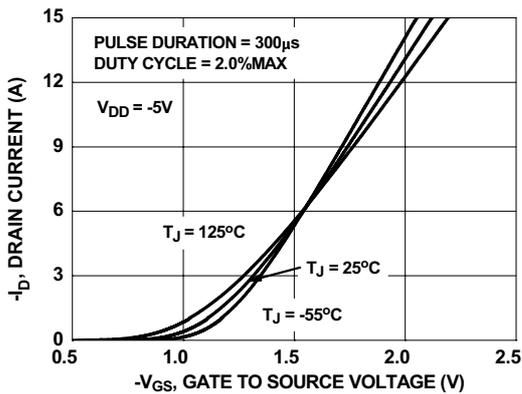
Figure 5. Transfer Characteristics
