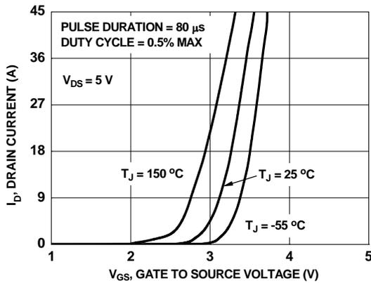
Figure 5. Transfer Characteristics
