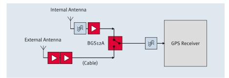
GPS receiver with 2nd external antenna
