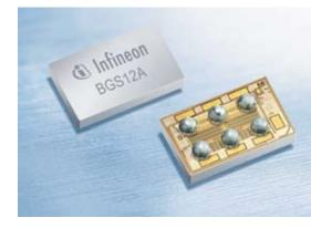
THE BGS12A is Infineon's first product in its new Radio Frequency (RF) switch family. The BGS12A is a general purpose Single-Pole, Double-Throw (SPDT) RF switch, designed for power levels of up to 2odBm, with a P-1dB above 3odBm.
