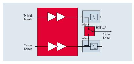
Power detection switch used in Dual Band Power Amplifier
