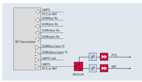
UMTS-multiband application with interstage switch
