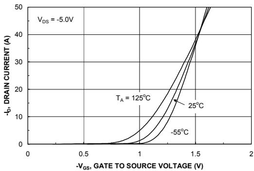
Figure 5. Transfer Characteristics.
