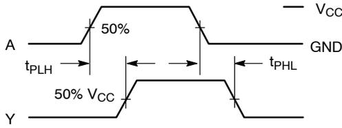
Figure 3. Switching Waveforms
