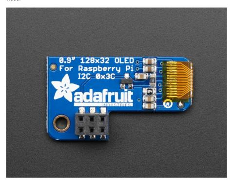
Comes completely pre-assembled and tested so you don't need to do anything but plug it in and install our Python code! Works with any Raspberry Pi computer, including the original Pi 1, B+, Pi 2, Pi 3 and Pi Zero.
