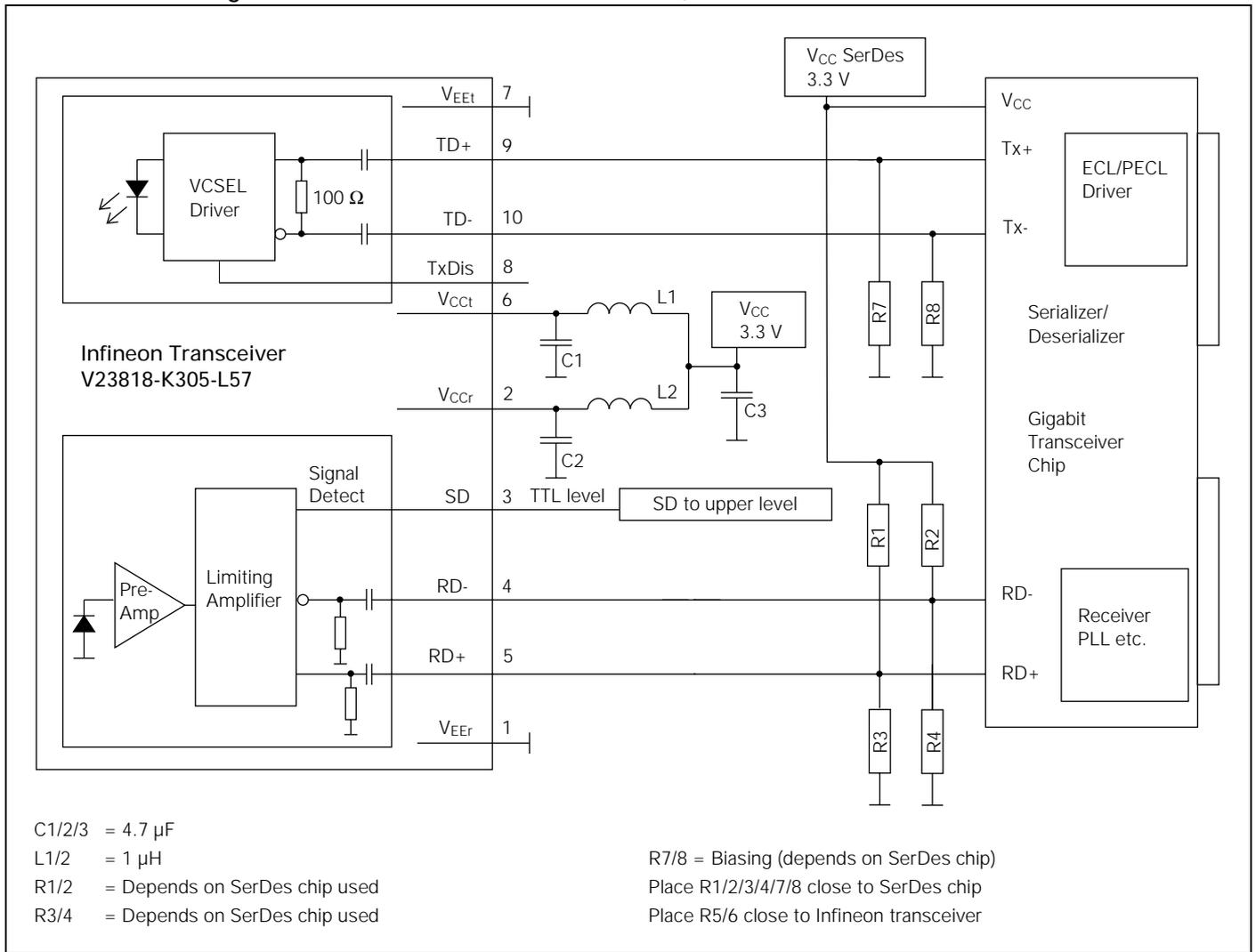
Values of R1/2/3/4 may vary as long as proper 50 Ω termination to V<sub>EE</sub> or 100 Ω differential is provided. The power supply filter-
