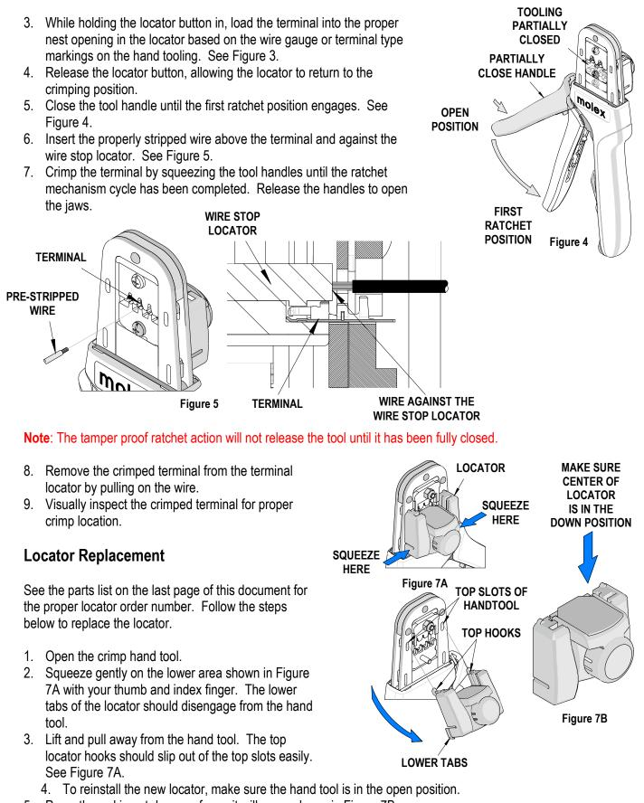
5. Press the red insert down as far as it will go as shown in Figure 7B.
