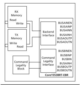
Figure 5 • Using Internal FPGA Memory Blocks
