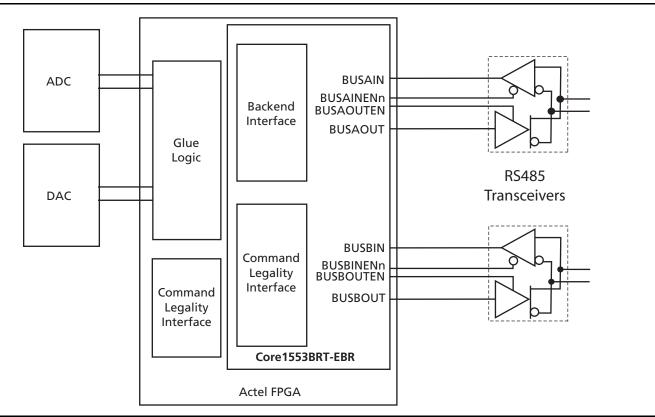
Figure 10 • Typical Non-Memory-Based RT System
