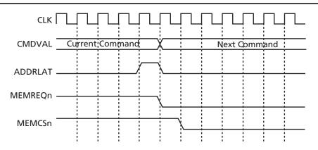
**Note:** This figure shows worst-case timing when a second 1553EBR command arrives as the core starts a backend transfer and MEMGNTn is held low.
