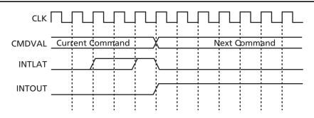
**Note:** This figure shows worst-case timing when a second 1553EBR command arrives as the core asserts an interrupt request. Also, INTLAT may be active for several clock cycles prior to INTOUT.
