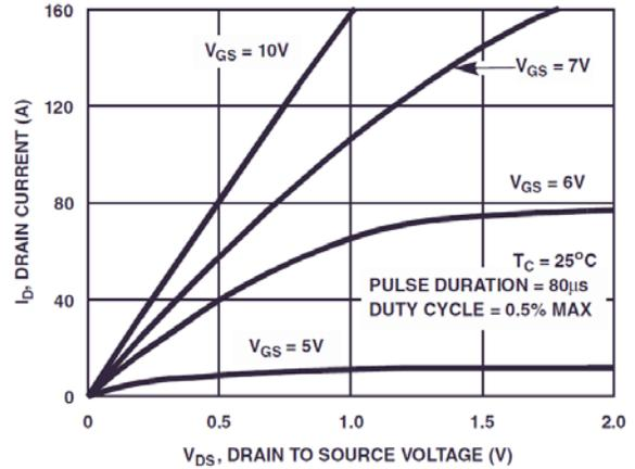
**Figure 8. Saturation Characteristics**
