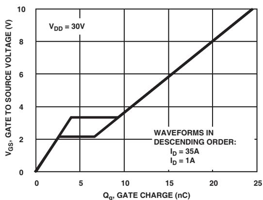
**Figure 14. Gate Charge Waveforms for Constant Gate Current**
