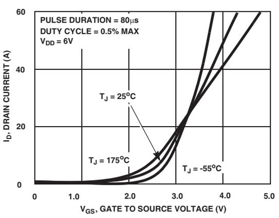
**Figure 7. Transfer Characteristics**
