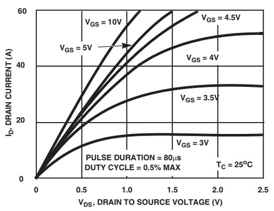
**Figure 8. Saturation Characteristics**
