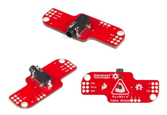
**Description:** The MyoWare Muscle Sensor is now designed to be wearable, allowing you to attach biomedical sensor pads directly to the board itself. However, there still may be cases where you want to mount the sensor pads away from the other hardware; this is where the MyoWare Cable Shield comes in. This shield provides a 3.5mm jack where you can attach a three-electrode sensor cable, allowing you to test and use the MyoWare Muscle Sensor without actually attaching it to your person.
