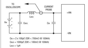
Figure 2. Measuring Input Ripple Current
