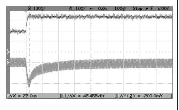
Step Load Transient Response (Vin=24V, Vout=12V, Cload=0, lout=3A to 1.5A) Trace 2=Vout, 100 mV/div. Trace 4=lout, 1A/div.
