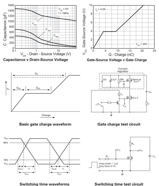
Switching time test circuit
