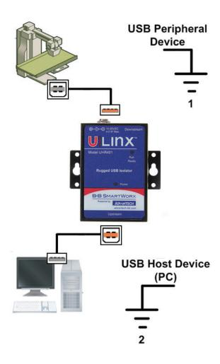
For optimum isolation the computer/host and the connected device should not use the same ground.
