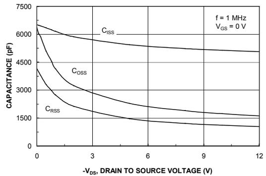
Figure 8. Capacitance Characteristics.
