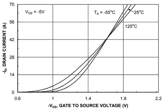
Figure 5. Transfer Characteristics.
