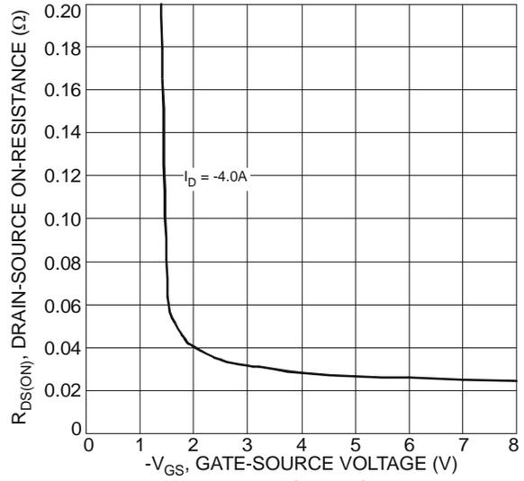
Fig. 4 Typical Drain-Source On-Resistance vs. Gate-Source Voltage
