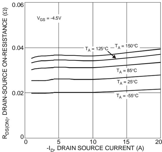
Fig. 5 Typical On-Resistance vs. Drain Current and Temperature
