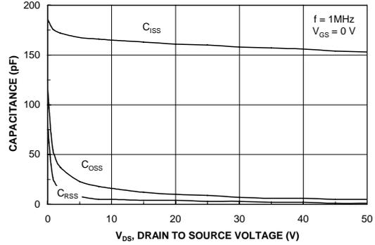
Figure 8. Capacitance Characteristics.
