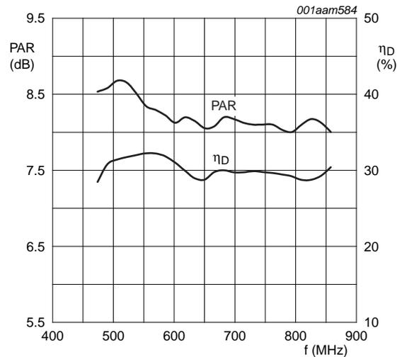
$P_{L(AV)} = 110\text{ W}$ ;  $V_{DS} = 50\text{ V}$ ;  $I_{Dq} = 1.3\text{ A}$ ; measured in a common source broadband test circuit as described in Section 8.
