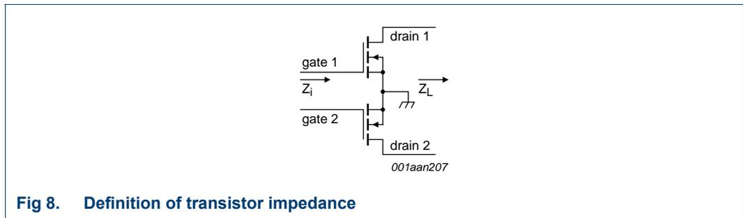
Fig 8. Definition of transistor impedance
