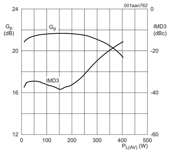
$V_{DS} = 50 \text{ V}$ ;  $I_{Dq} = 1.3 \text{ A}$ ; measured in a common source narrowband 860 MHz test circuit.
