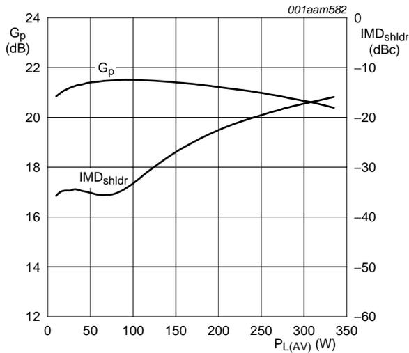
$V_{DS} = 50\text{ V}$ ;  $I_{Dq} = 1.3\text{ A}$ ; measured in a common source narrowband 860 MHz test circuit.
