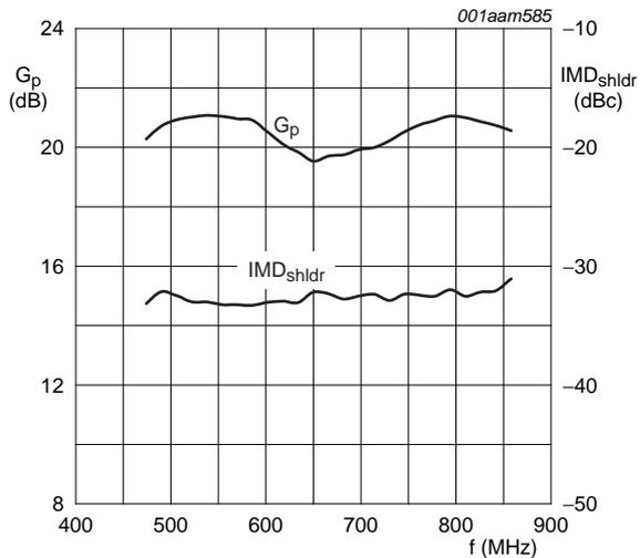
$P_{L(AV)} = 110\text{ W}$ ;  $V_{DS} = 50\text{ V}$ ;  $I_{Dq} = 1.3\text{ A}$ ; measured in a common source broadband test circuit as described in Section 8.
