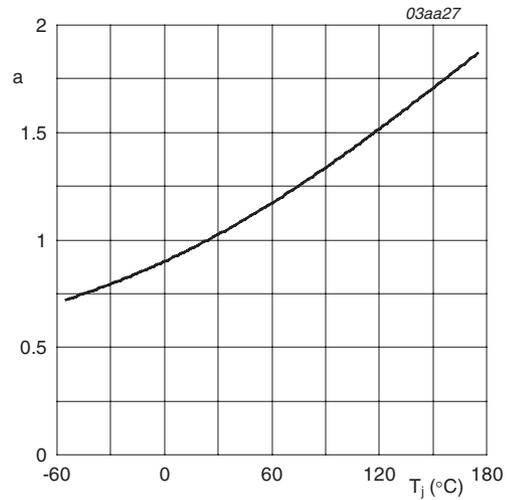
$$a = \frac{R_{DSon}}{R_{DSon(25^\circ\text{C})}}$$
