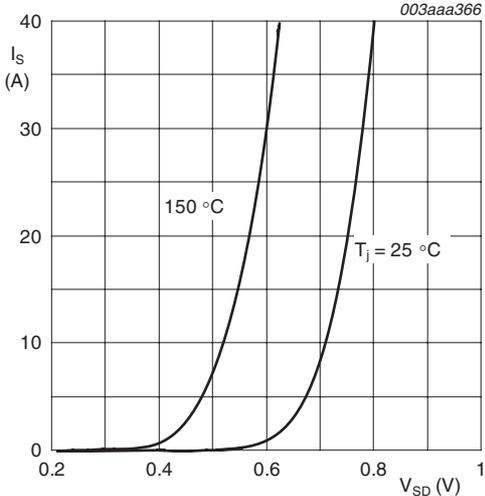
$T_j = 25^\circ\text{C}$  and  $150^\circ\text{C}; V_{GS} = 0\text{V}$
