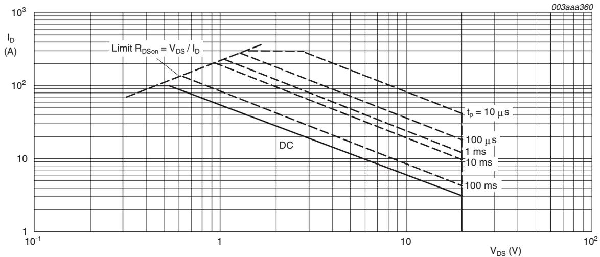
$$T_{mb} = 25^\circ\text{C}; I_{DM} \text{ is single pulse}; V_{GS} = 10\text{V}$$
