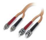
Assembled FO cable, zip cord cable, multi-mode fiberglass 62.5/125 µm, OM1, plug: FSMA/B-FOC (ST), degree of protection: IP20, for installation in cable ducts or control cabinets
