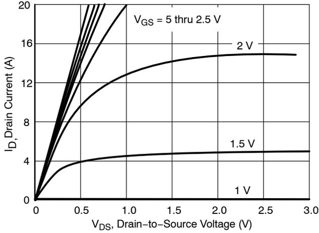
Figure 1. Output Characteristics
