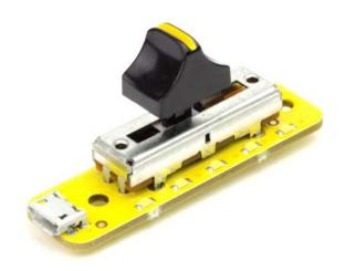
The Slider module is a slide potentiometer which has five bright white LEDs that illuminate as the slider is moved. It's perfect for using as a synth controller or for controlling the speed of your robot.
