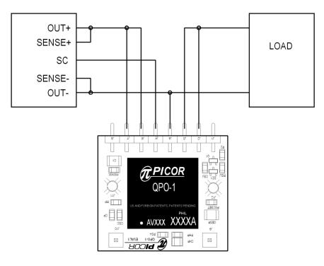
Figure 4 – Evaluation board in SC configuration.
