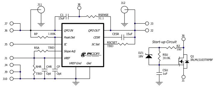
Figure 3 – Evaluation board schematic.
