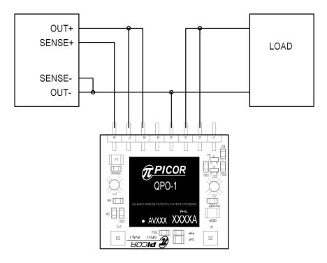
**Figure 5** – Evaluation board in Remote Sense configuration.
