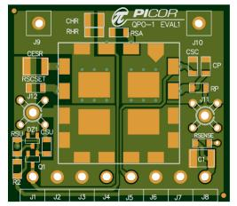
Figure 1 - Top View of Evaluation Board.
