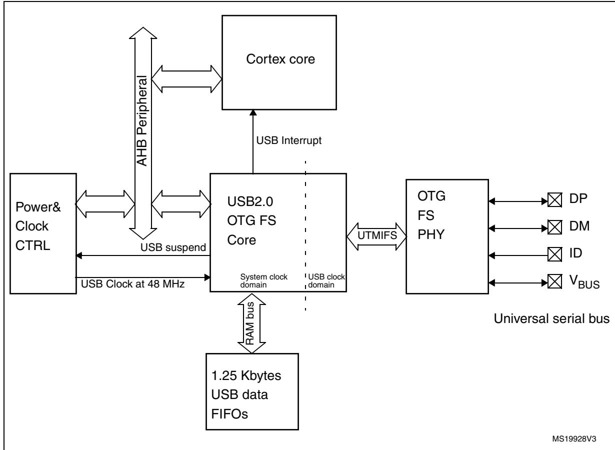
Figure 489. OTG high-speed block diagram
