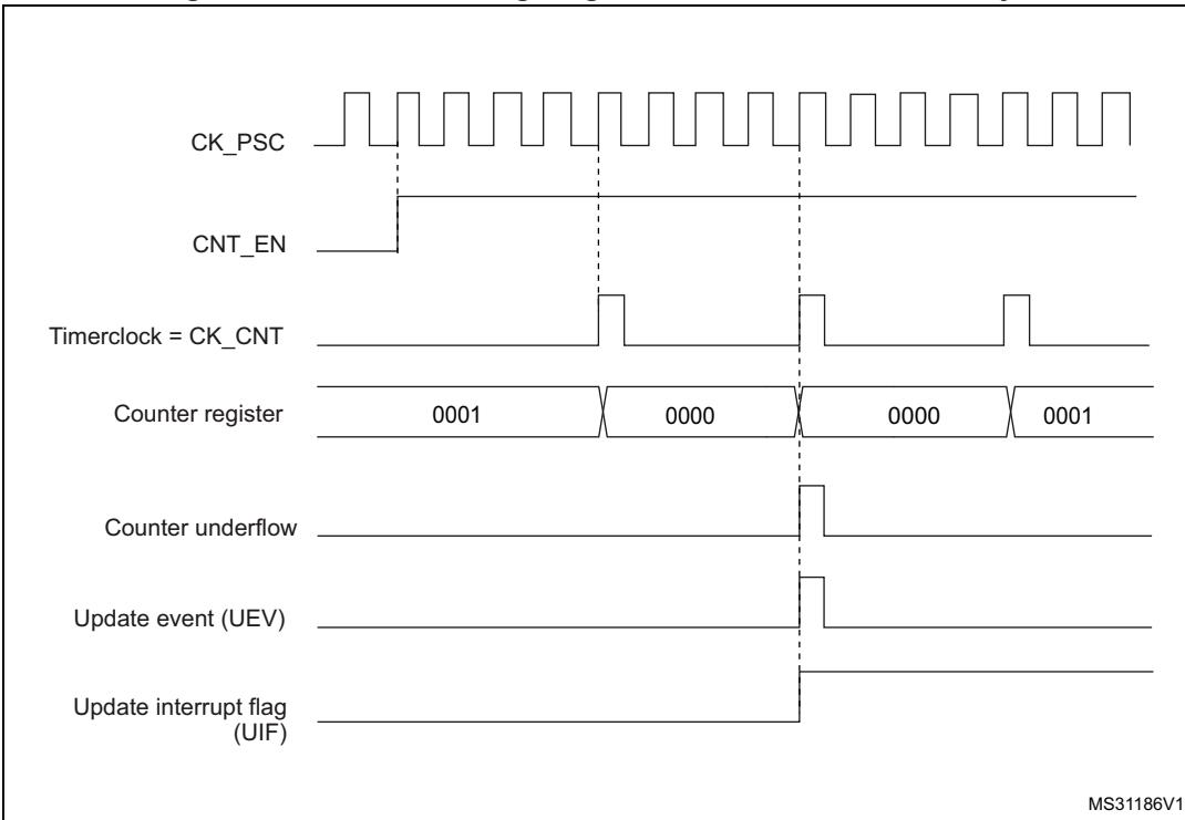
Figure 190. Counter timing diagram, internal clock divided by N
