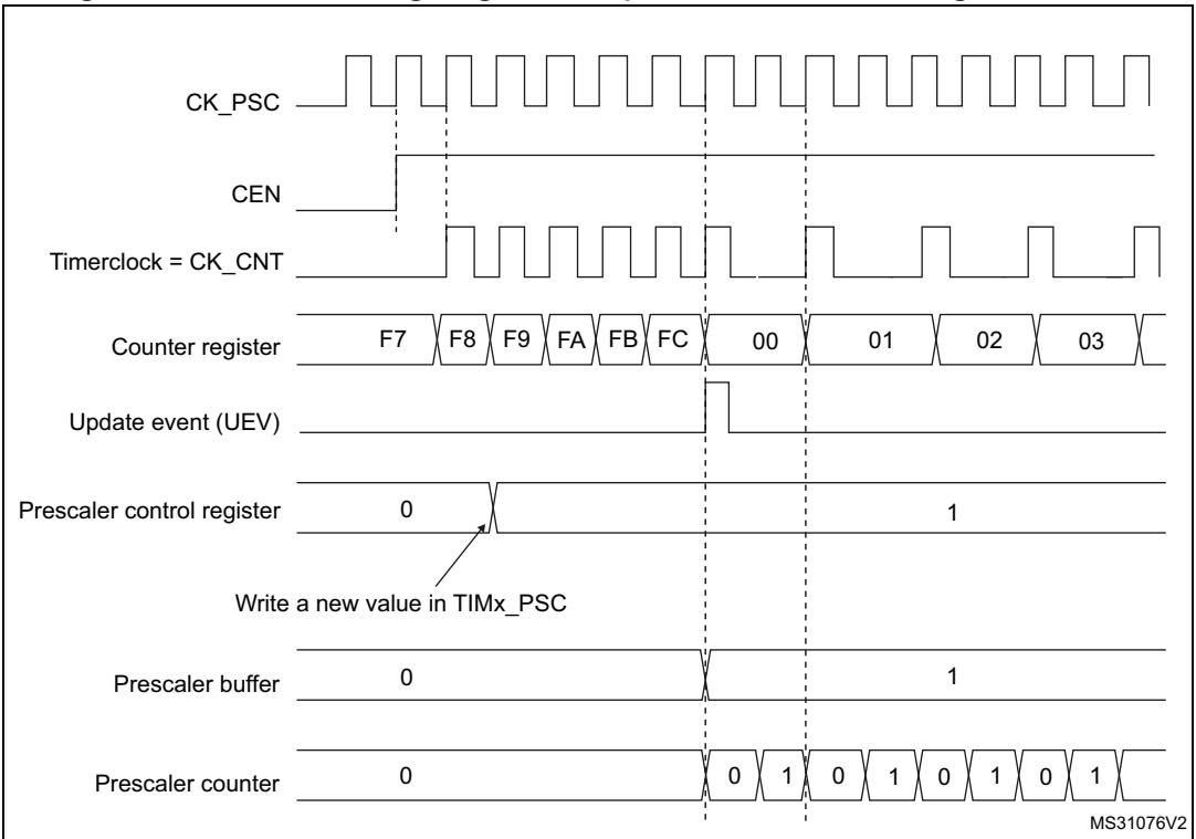
**Figure 288. Counter timing diagram with prescaler division change from 1 to 4**
