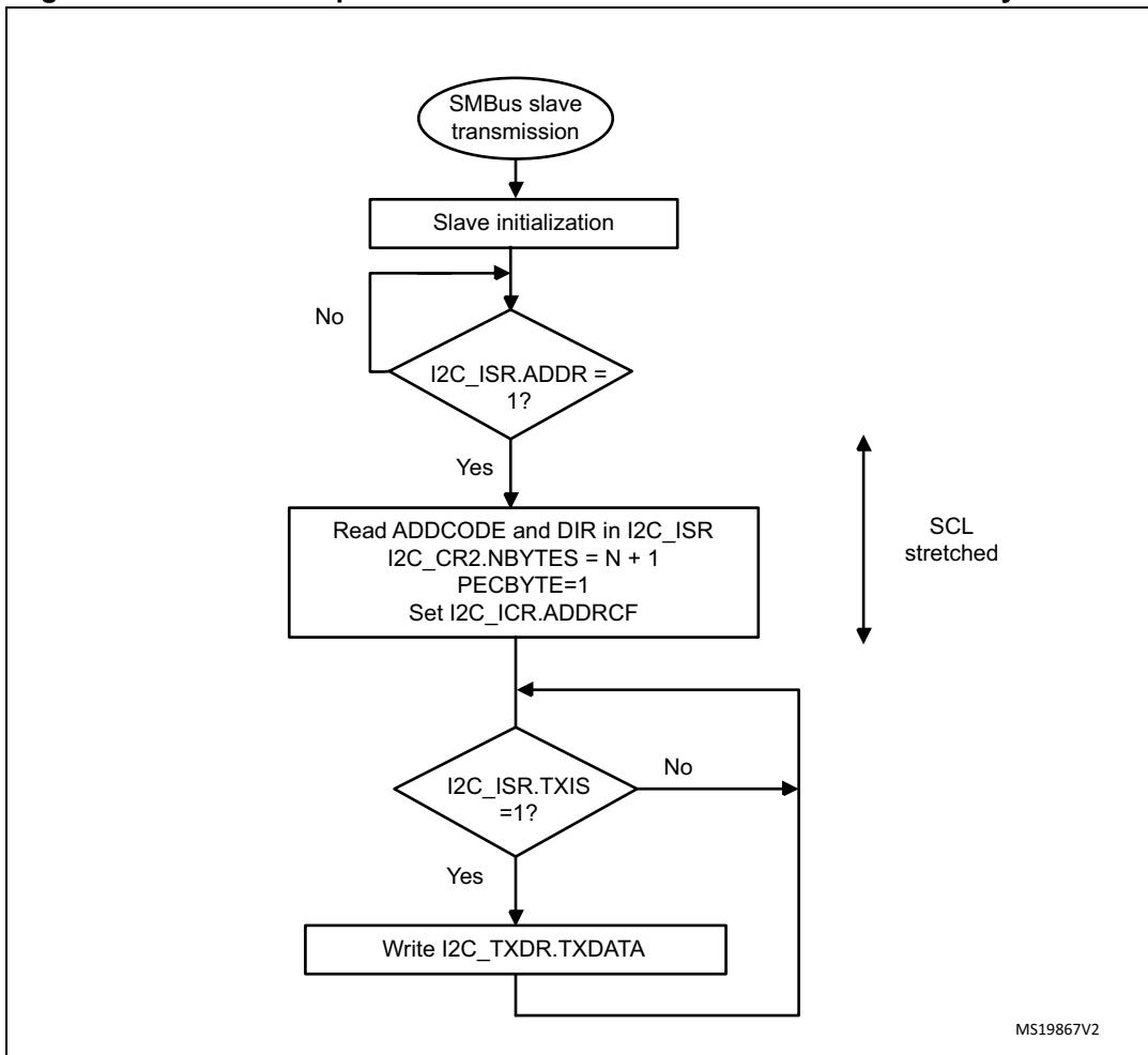
Figure 355. Transfer bus diagrams for SMBus slave transmitter (SBC=1)
