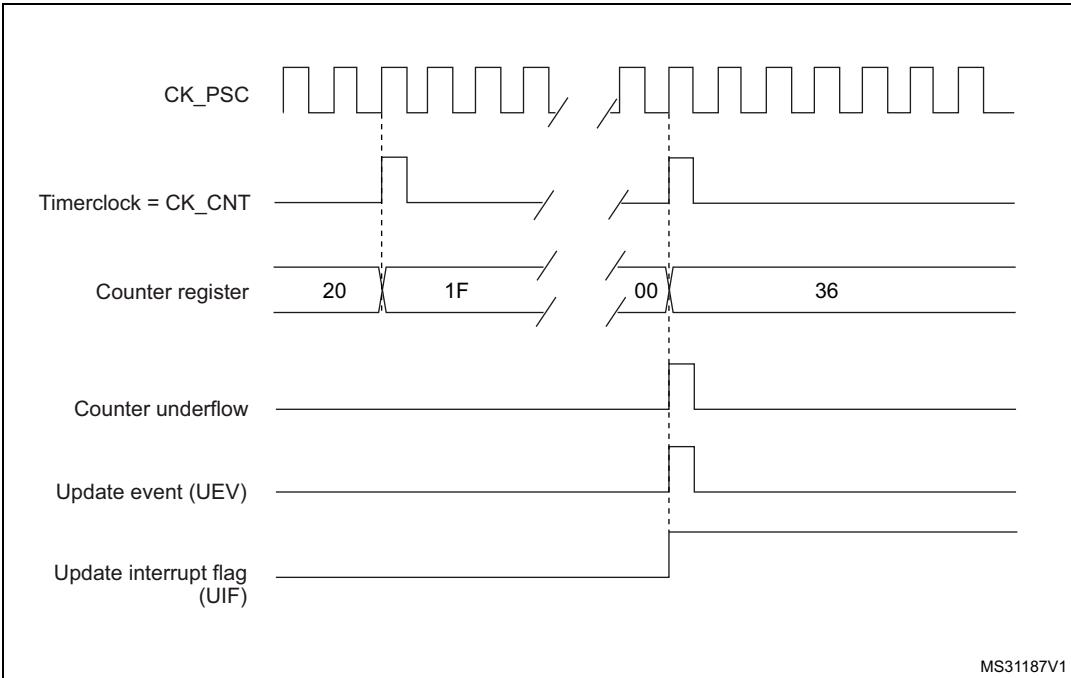
**Figure 249. Counter timing diagram, Update event when repetition counter is not used**
