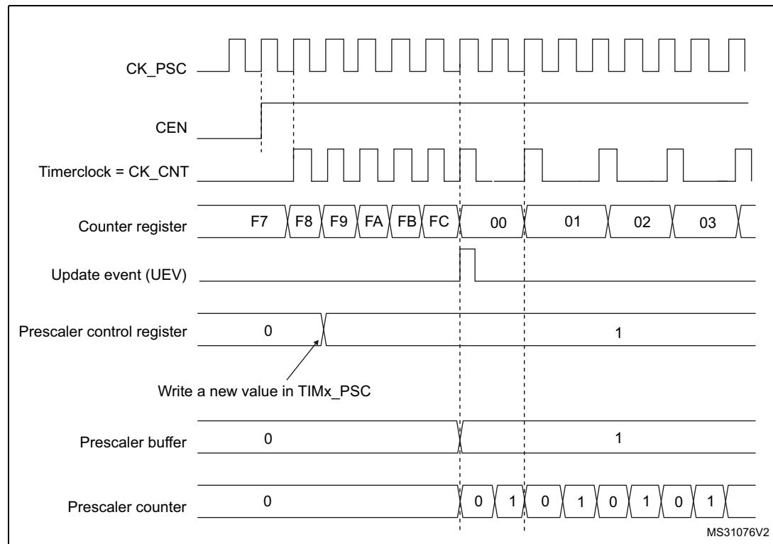
**Figure 311. Counter timing diagram with prescaler division change from 1 to 4**
