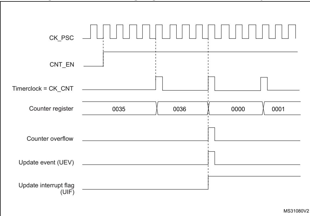
**Figure 184. Counter timing diagram, internal clock divided by N**
