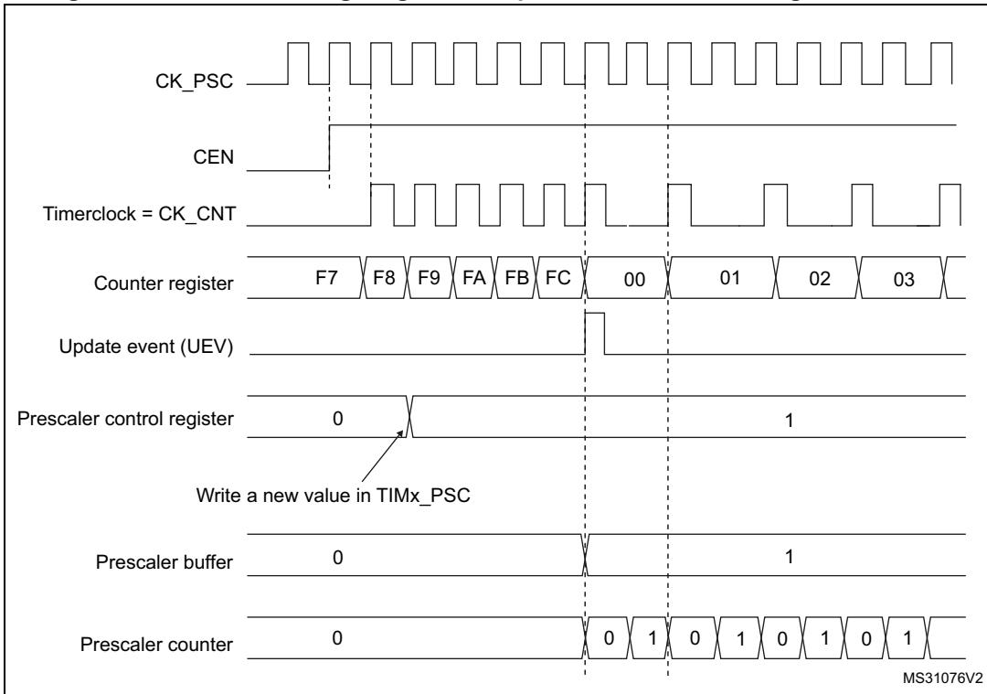
**Figure 180. Counter timing diagram with prescaler division change from 1 to 4**
