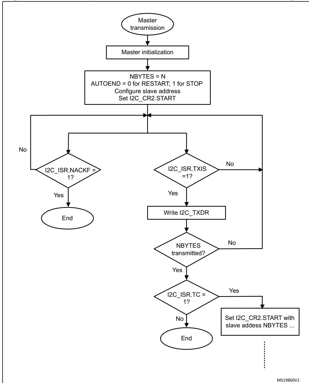
Figure 348. Transfer sequence flowchart for I2C master transmitter for N&gt;255 bytes
