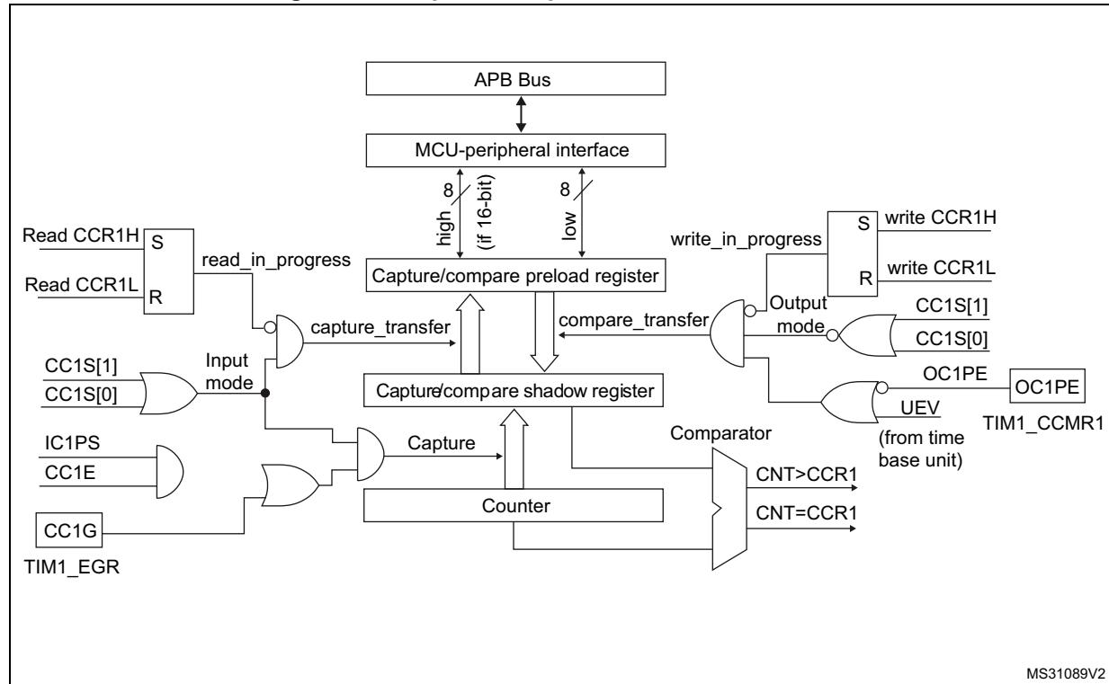
**Figure 207.** Output stage of capture/compare channel (channel 1, idem ch. 2 and 3)
