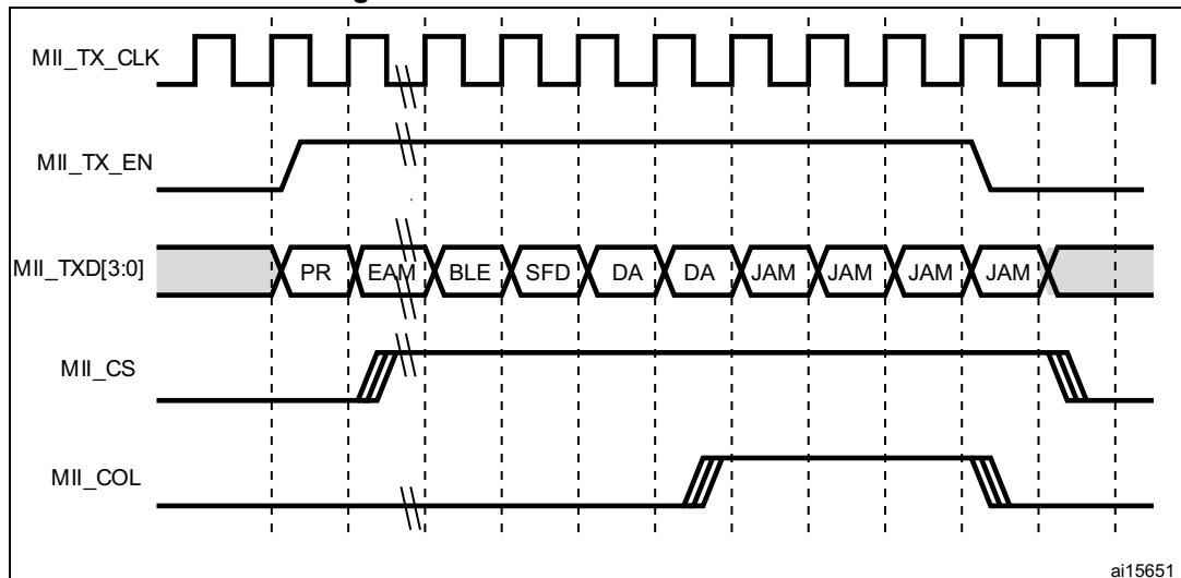
[Figure 535](#) shows a frame transmission in MII and RMII.
