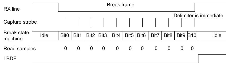
**Case 3: break signal long enough => break detected, LBDF is set**
