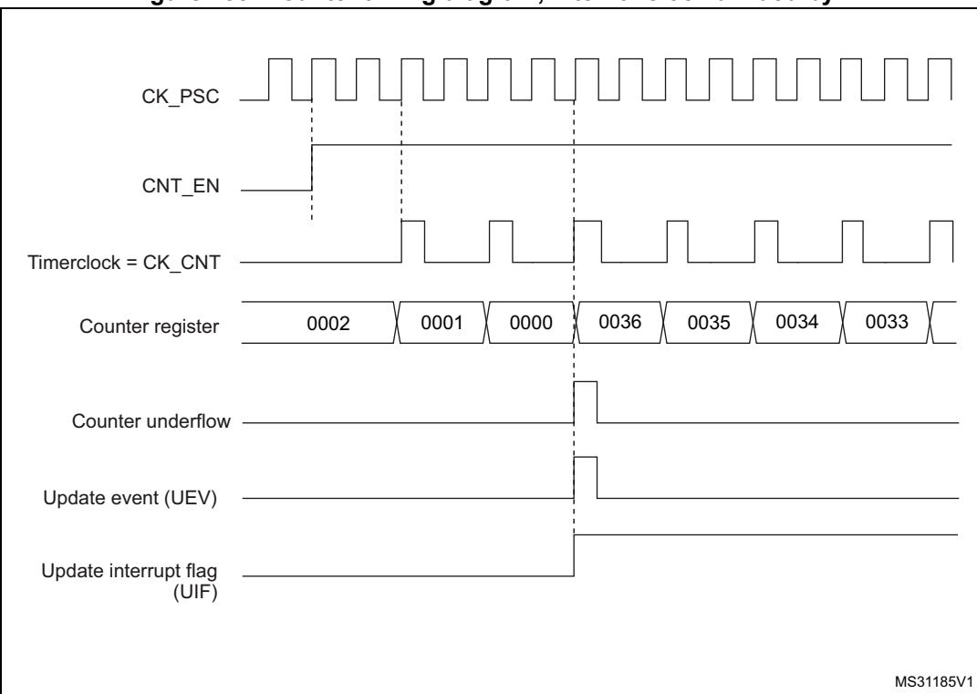
Figure 189. Counter timing diagram, internal clock divided by 4
