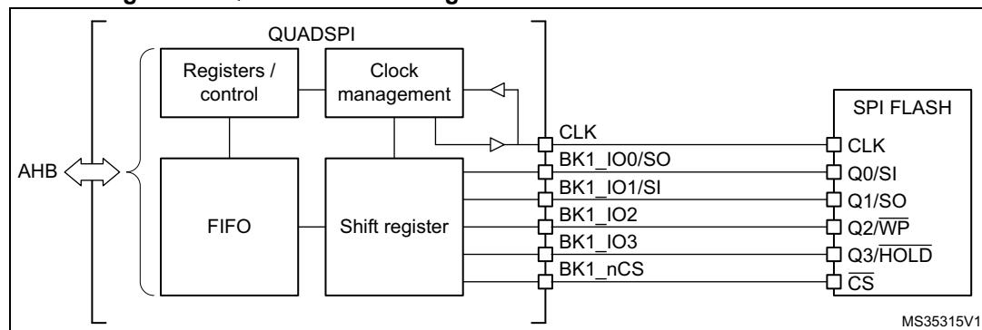
**Figure 62. QUADSPI block diagram when dual-flash mode is enabled**
