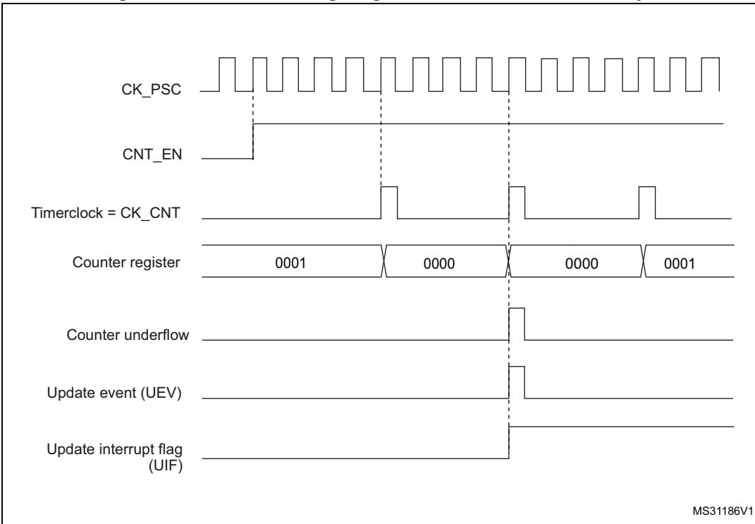
**Figure 248. Counter timing diagram, internal clock divided by N**
