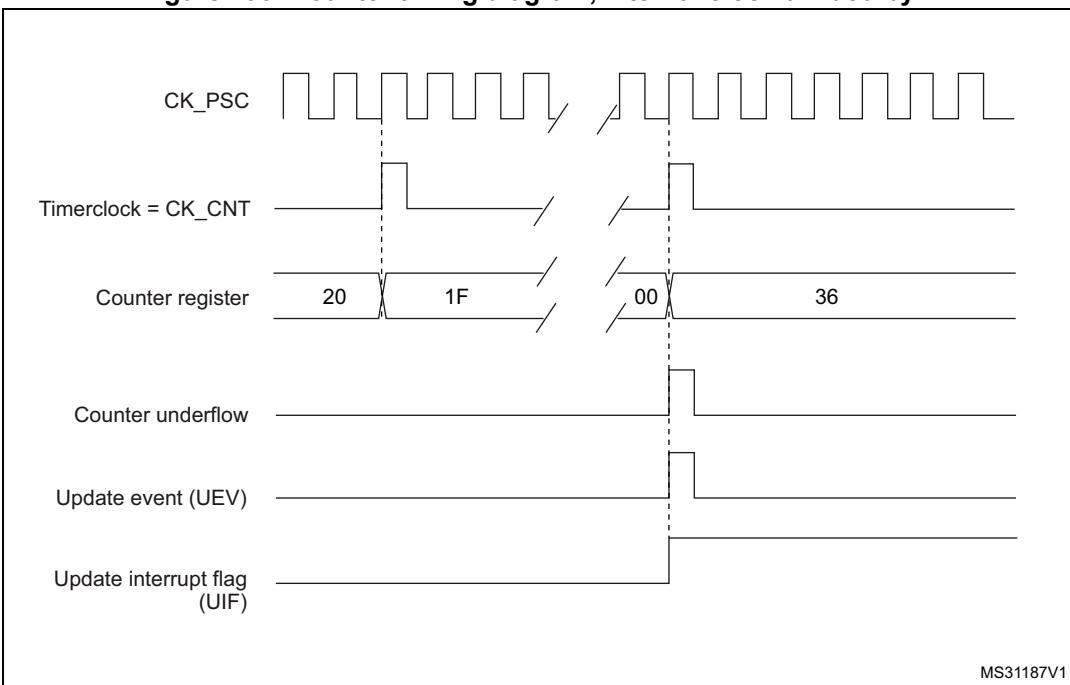
**Figure 191. Counter timing diagram, update event when repetition counter is not used**
