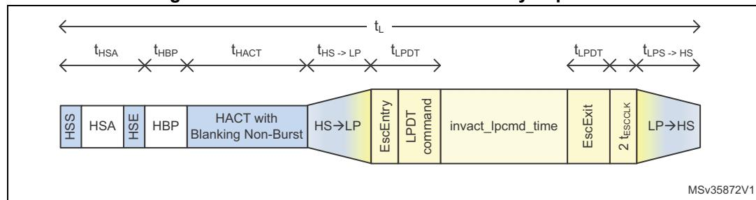
**Figure 142. VLPSIZE for Non-Burst with sync events**
