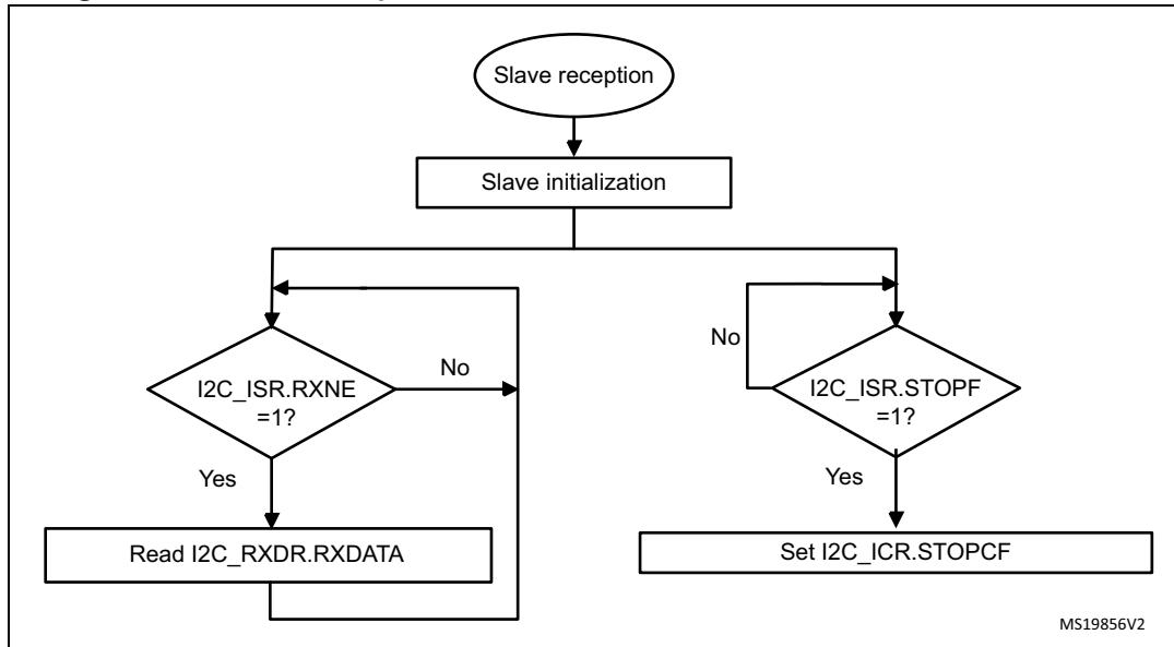
**Figure 342.** Transfer bus diagrams for I2C slave receiver
