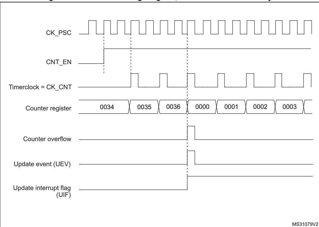
**Figure 314. Counter timing diagram, internal clock divided by 4**
