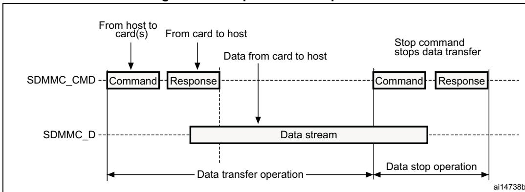
**Figure 462. Sequential write operation**
