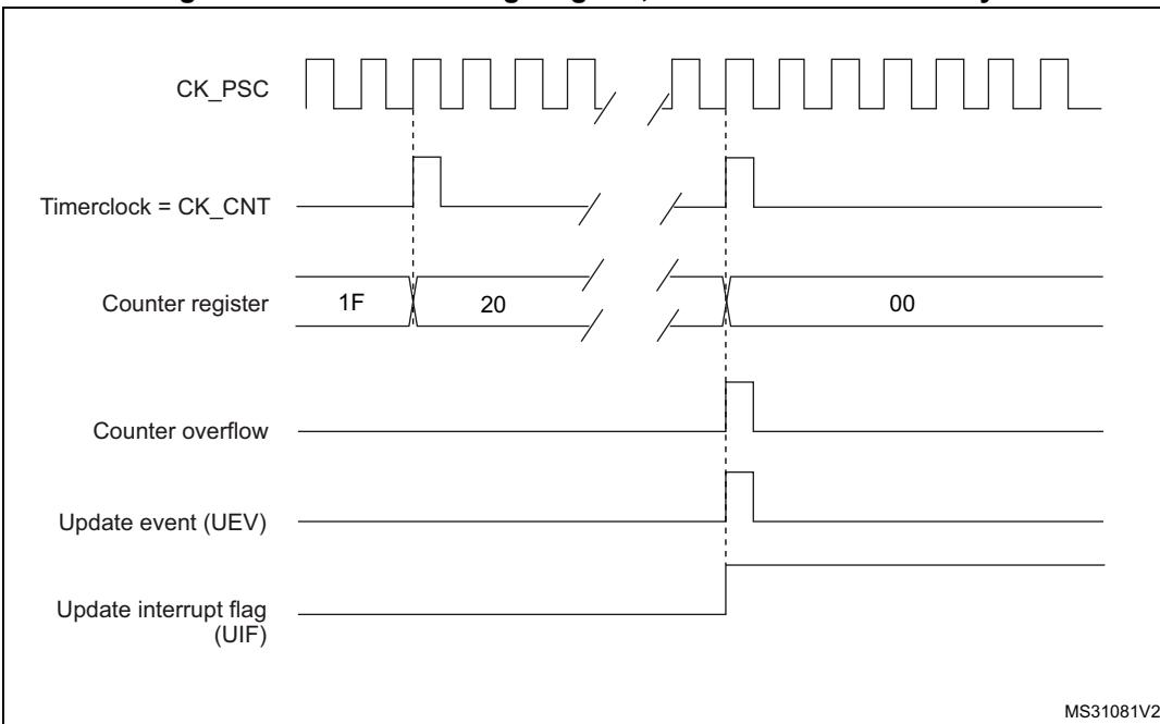
**Figure 293. Counter timing diagram, update event when ARPE=0 (TIMx\_ARR not preloaded)**
