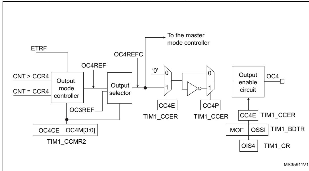
Figure 209. Output stage of capture/compare channel (channel 5, idem ch. 6)
