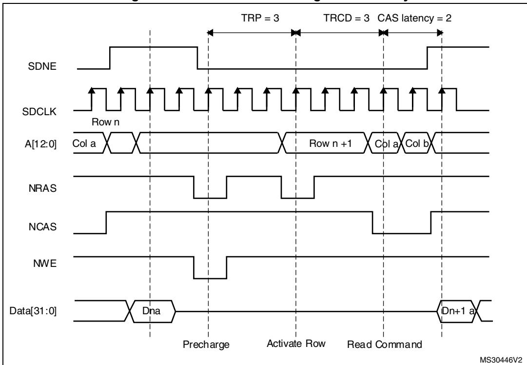
**Figure 58. Write access crossing row boundary**
