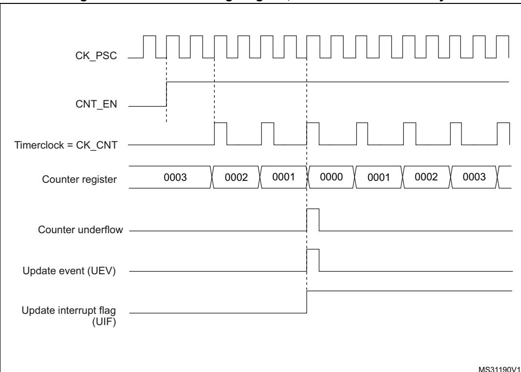
**Figure 252. Counter timing diagram, internal clock divided by 4, TIMx\_ARR=0x36**
