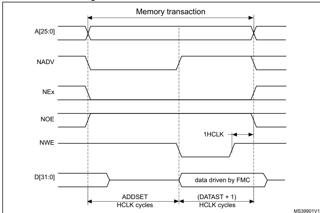
**Figure 40. ModeB write access waveforms**
