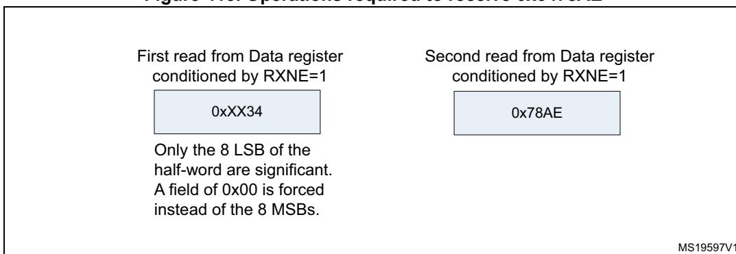
**Figure 416.** LSB justified 16-bit extended to 32-bit packet frame
