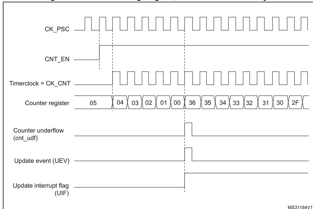
**Figure 246. Counter timing diagram, internal clock divided by 2**
