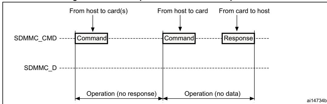
**Figure 459. (Multiple) block read operation**
