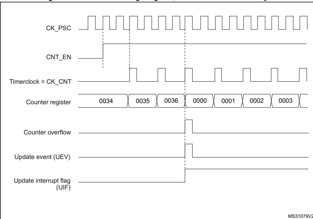
**Figure 291. Counter timing diagram, internal clock divided by 4**
