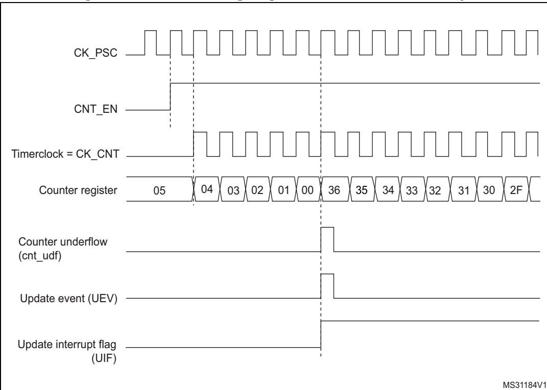
**Figure 188. Counter timing diagram, internal clock divided by 2**
