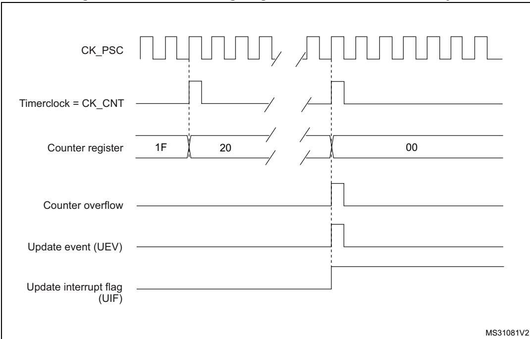
**Figure 243. Counter timing diagram, Update event when ARPE=0 (TIMx\_ARR not preloaded)**
