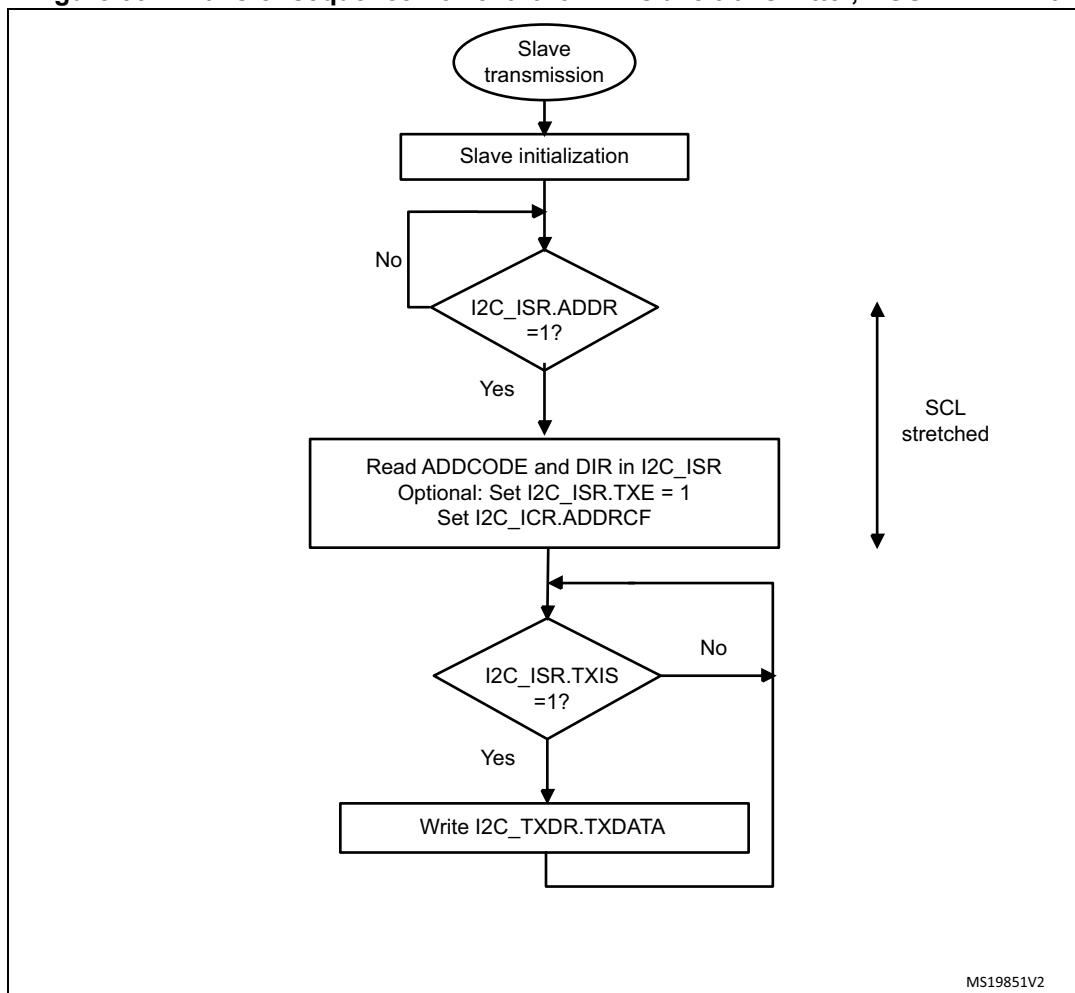
**Figure 338. Transfer sequence flowchart for I2C slave transmitter, NOSTRETCH=1**
