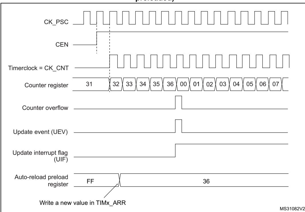
**Figure 294. Counter timing diagram, update event when ARPE=1 (TIMx\_ARR preloaded)**
