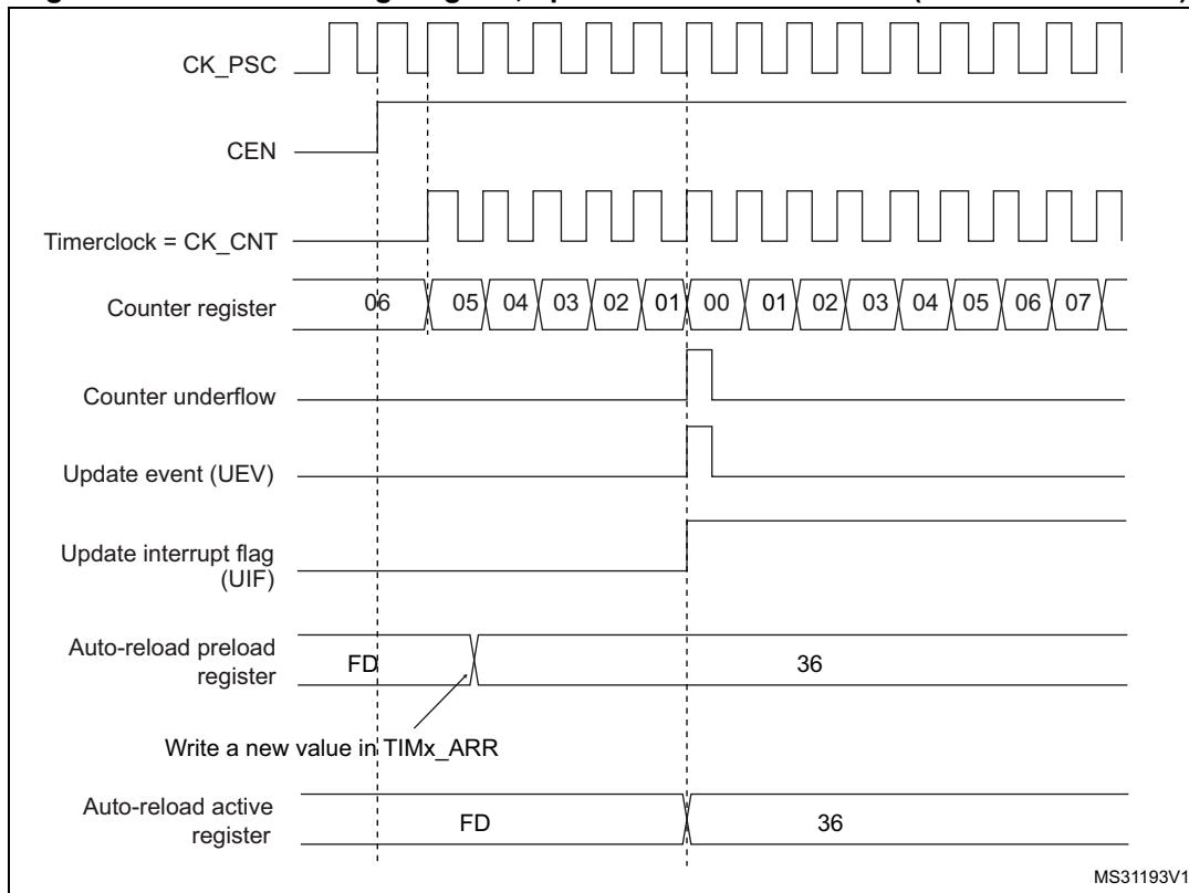
**Figure 197. Counter timing diagram, Update event with ARPE=1 (counter overflow)**
