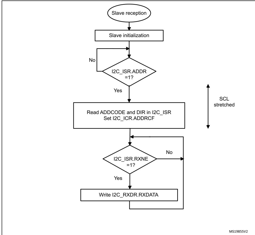
**Figure 341.** Transfer sequence flowchart for slave receiver with NOSTRETCH=1
