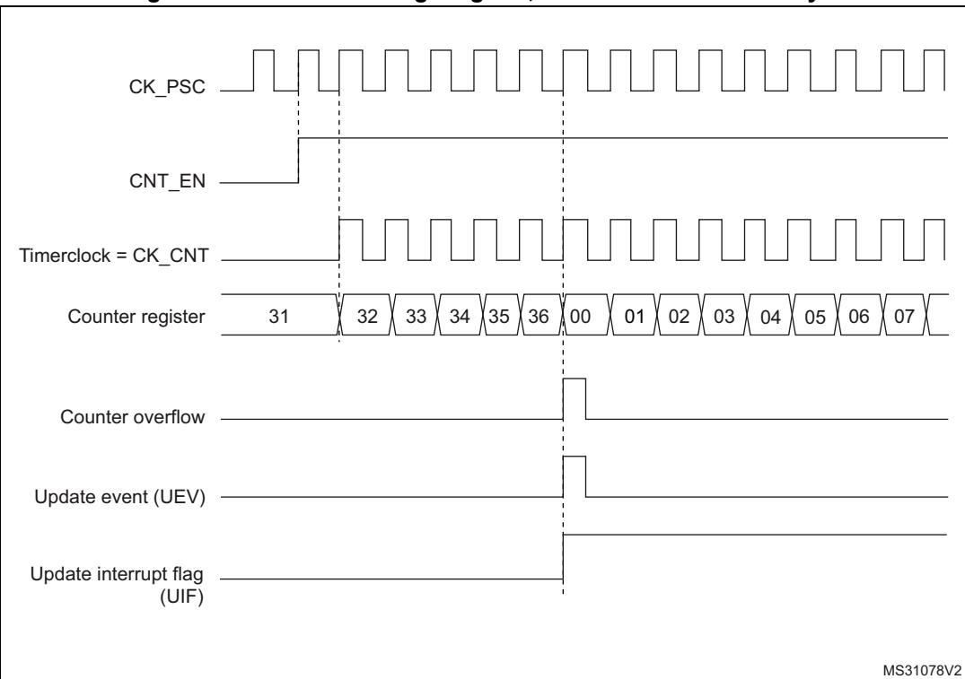
**Figure 182. Counter timing diagram, internal clock divided by 2**
