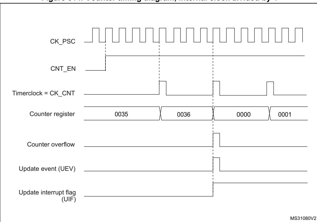
**Figure 315. Counter timing diagram, internal clock divided by N**
