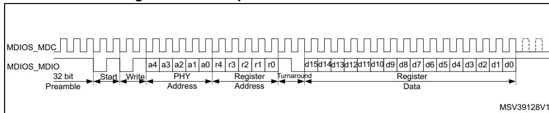
**Figure 457. MDIO protocol read frame waveform**
