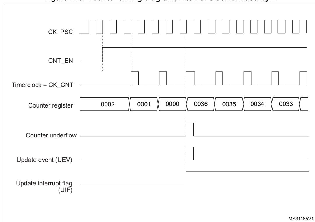
**Figure 247. Counter timing diagram, internal clock divided by 4**
