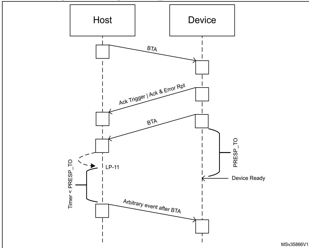
**Figure 134. Timing of PRESP\_TO after a Read Request (HS or LP)**
