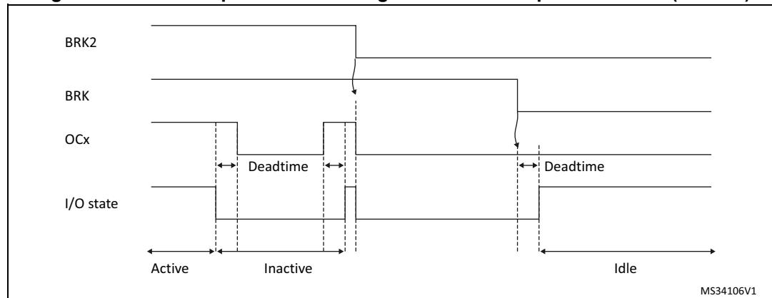
**Figure 223. PWM output state following BRK assertion (OSSI=0)**
