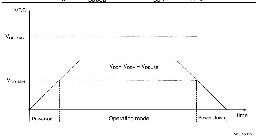
**Figure 6.  $V_{DDUSB}$  connected to external independent power supply**
