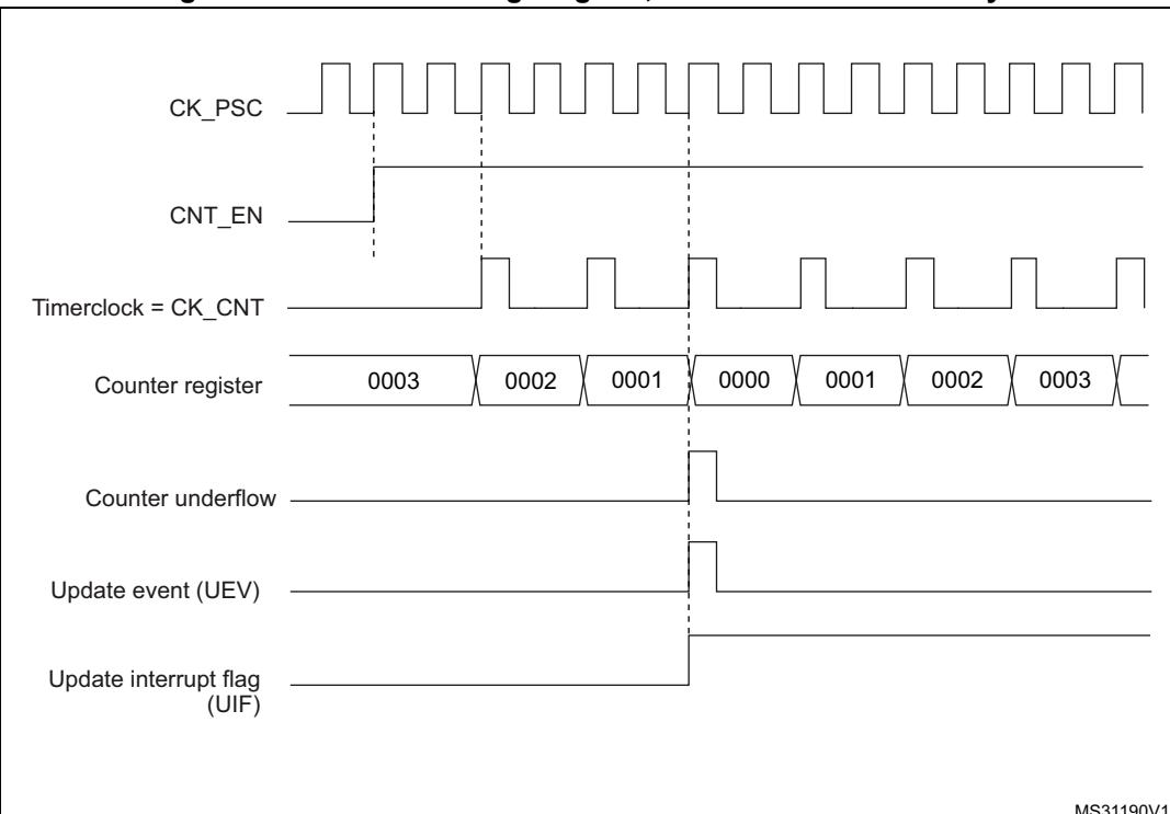
**Figure 194. Counter timing diagram, internal clock divided by 4, TIMx\_ARR=0x36**
