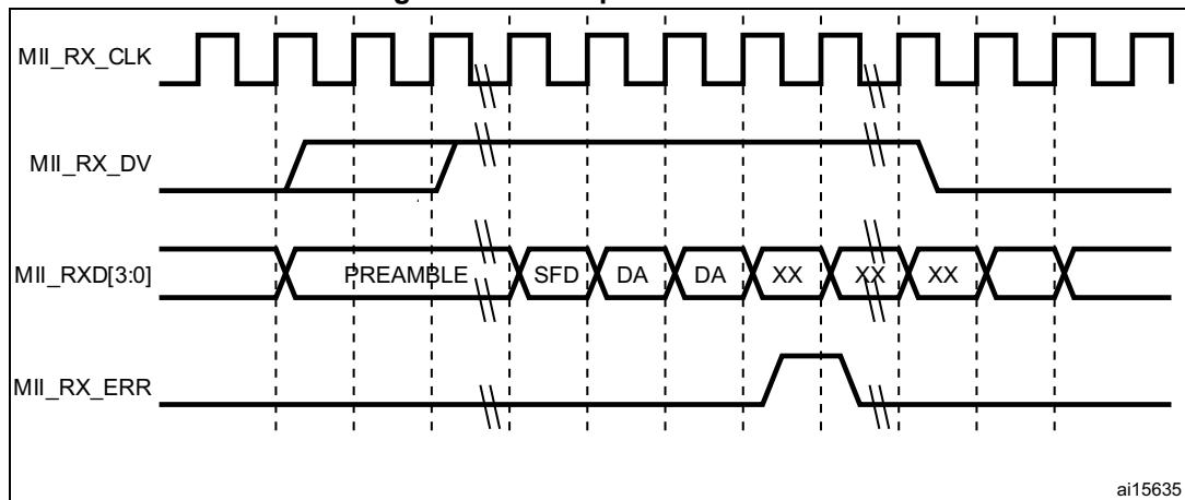
**Figure 539. Reception with false carrier indication**
