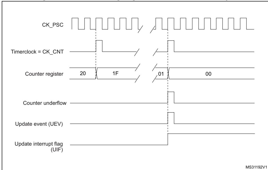
**Figure 196. Counter timing diagram, update event with ARPE=1 (counter underflow)**
