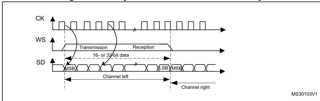
**Figure 413. LSB justified 24-bit frame length**
