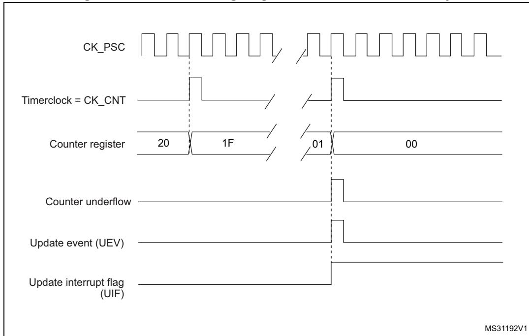
**Figure 254. Counter timing diagram, Update event with ARPE=1 (counter underflow)**
