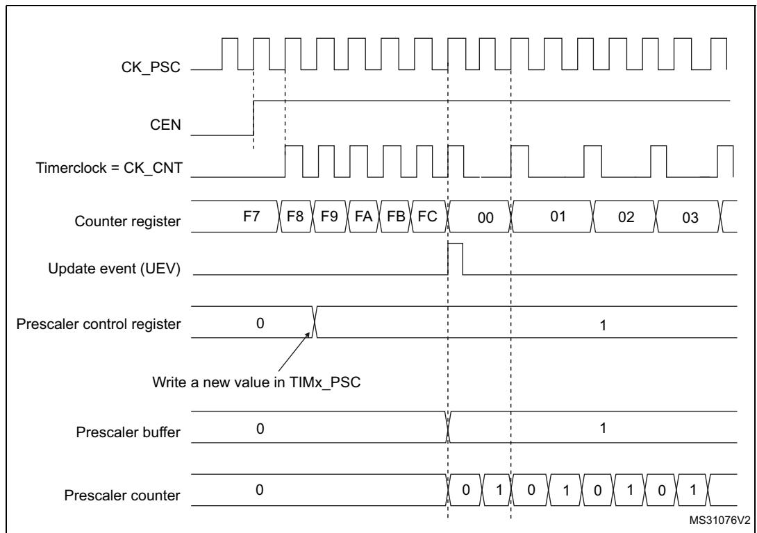
**Figure 238. Counter timing diagram with prescaler division change from 1 to 4**
