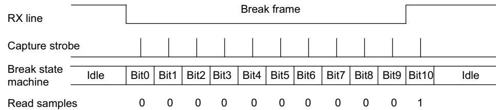
**Case 2: break signal just long enough => break detected, LBDF is set**
