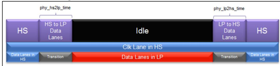
**Figure 147. Clock lane and data lane in LP**
