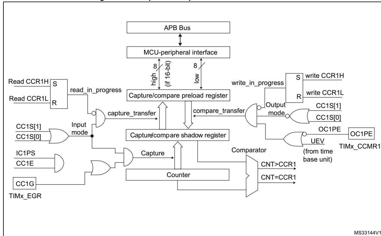
Figure 263. Output stage of capture/compare channel (channel 1)
