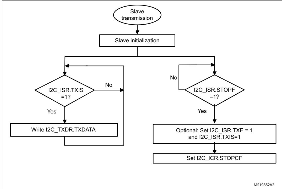
Figure 339. Transfer bus diagrams for I2C slave transmitter
