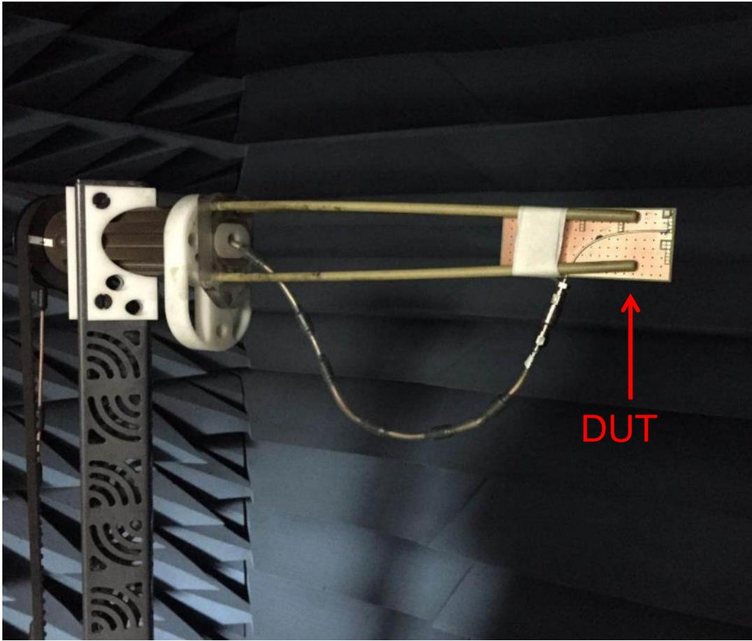
**FIGURE4.1.3 ANTENNA LOADED WITH OTA CHAMBER**
