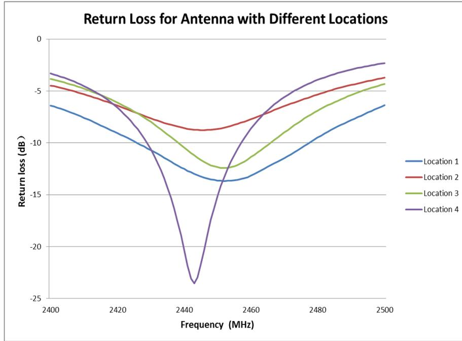
**FIGURE 7.3.2 RETURN LOSS COMPARISON AT 2.4 GHZ BAND AT FOUR LOCATIONS**
