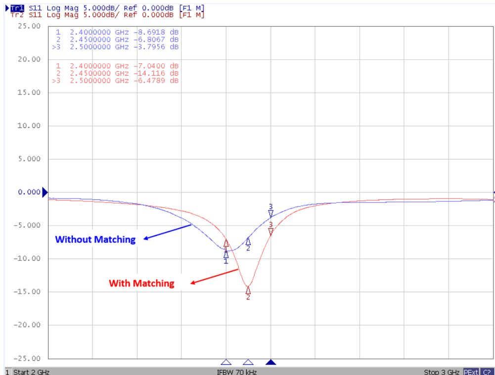
**FIGURE 6.2 RETURN LOSS COMPARISON WITH AND WITHOUT MATCHING ON REFERENCE PCB GROUND SIZE AT REFERENCE LOCATION**
