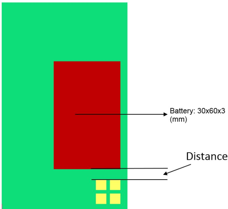
**FIGURE 7.2.1 BATTERY FIXED ON REFERENCE PCB**
