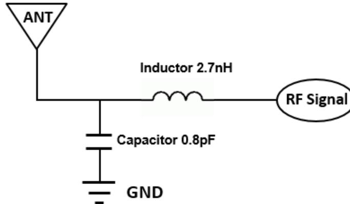
**FIGURE 6.1 RECOMMENDED MATCHING CIRCUIT FOR 2.4GHZ BAND**
