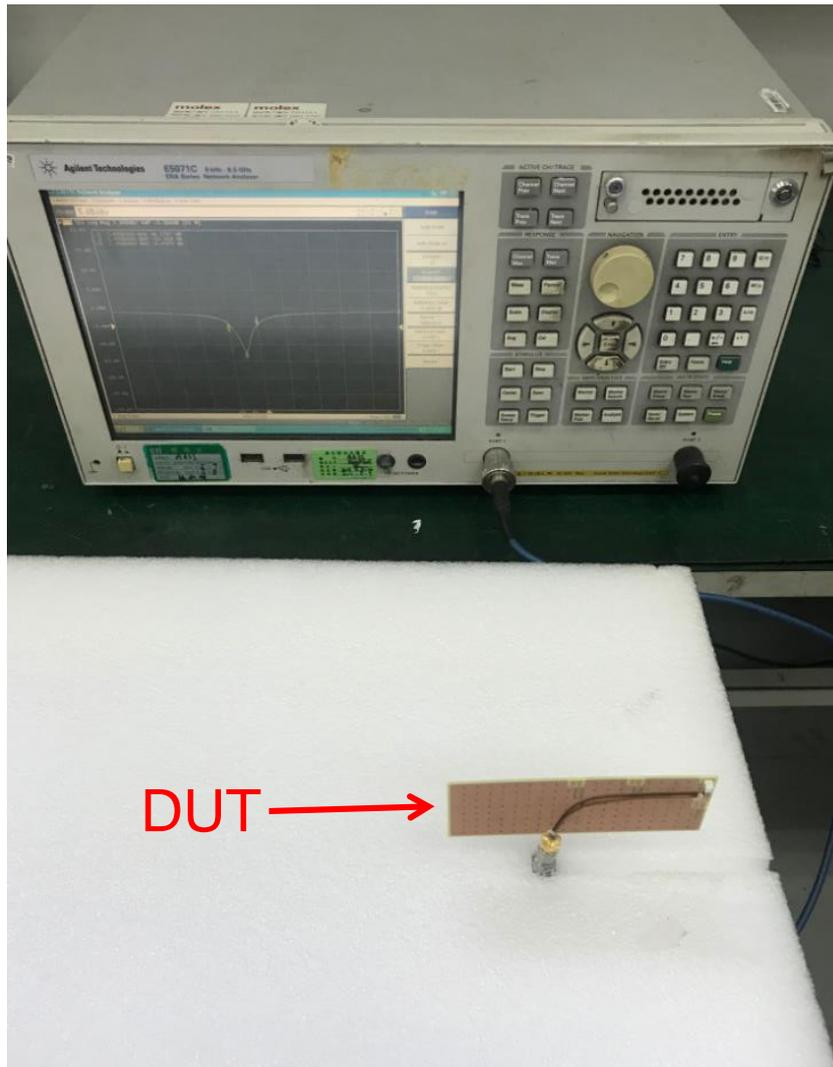
**FIGURE 4.1.2 ANTENNA LOADED WITH VNA**
