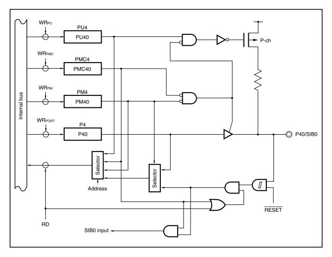
Figure 4-17. Block Diagram of P40 Pin
