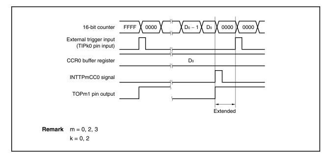
If the trigger is detected immediately before the INTTPmCC0 signal is generated, the INTTPmCC0 signal is not generated. The 16-bit counter is cleared to 0000H, the TOPm1 pin is asserted, and the counter continues counting. Consequently, the inactive period of the PWM waveform is shortened.
