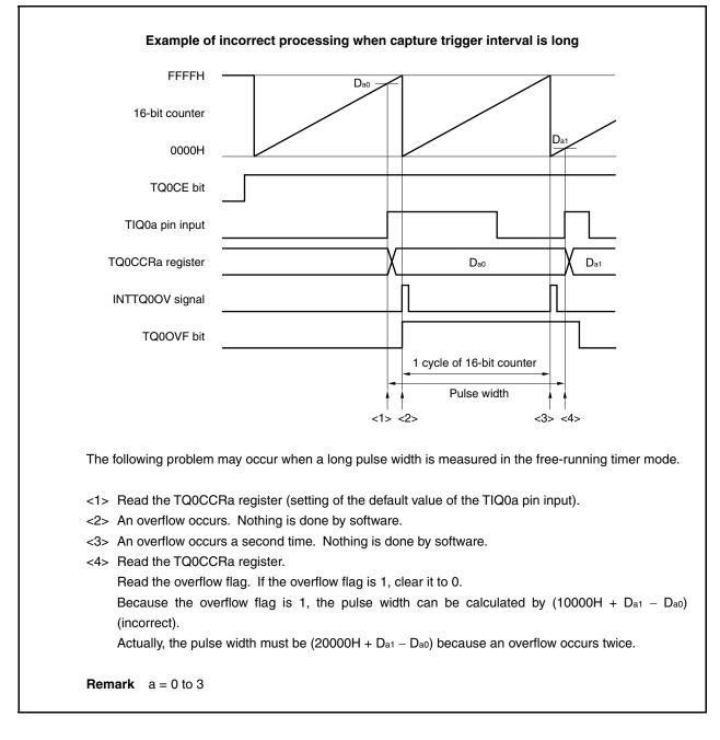
If an overflow occurs twice or more when the capture trigger interval is long, the correct pulse width may not be obtained.
