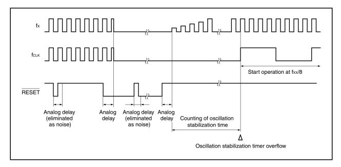
Figure 16-1. Timing of Reset Operation by RESET Pin Input
