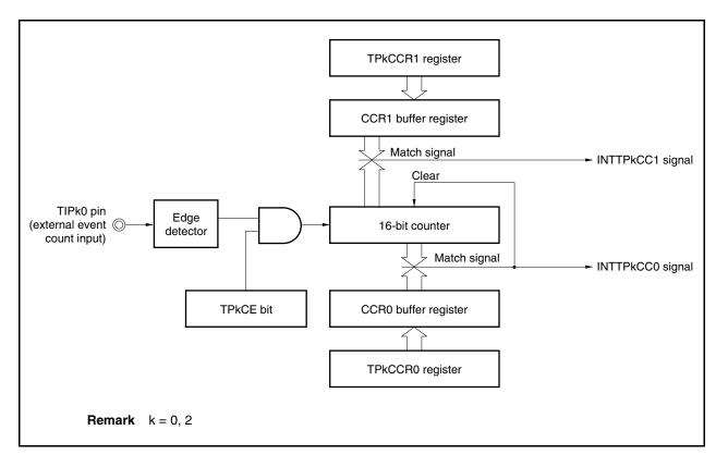
Figure 6-20. Configuration of TPkCCR1 Register
