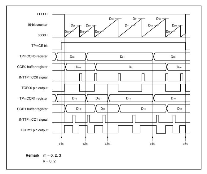
Figure 6-34. Software Processing Flow in PWM Output Mode (1/2)
