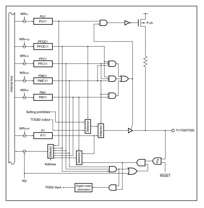
Figure 4-6. Block Diagram of P11 Pin
