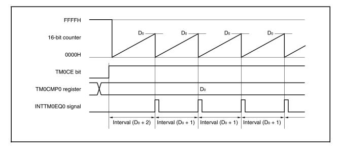
When the TM0CE bit is set to 1, the value of the 16-bit counter is cleared from FFFFH to 0000H in synchronization with the count clock, and the counter starts counting.
