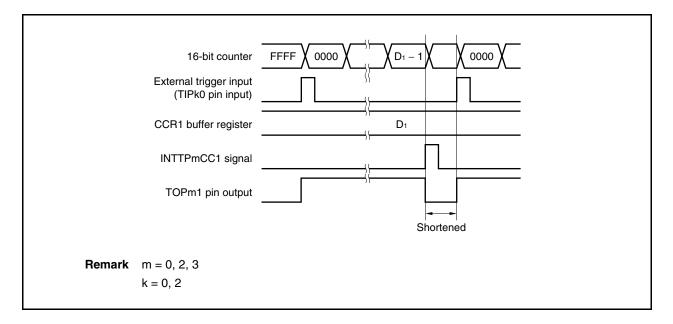
If the trigger is detected immediately before the INTTPmCC1 signal is generated, the INTTPmCC1 signal is not generated, and the 16-bit counter is cleared to 0000H and continues counting. The output signal of the TOPm1 pin remains active. Consequently, the active period of the PWM waveform is extended.
