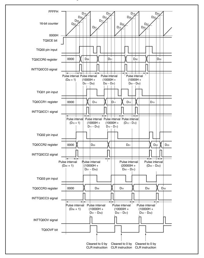
When executing pulse width measurement in the free-running timer mode, four pulse widths can be measured with one channel.
