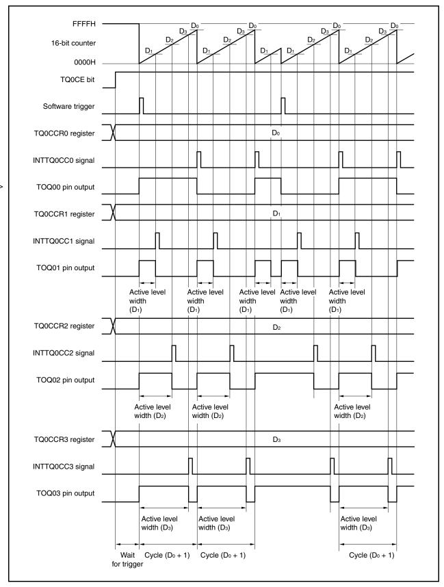
Figure 7-23. Basic Timing in External Trigger Pulse Output Mode
