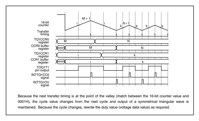
Figure 9-29. Example of Rewriting TQ1CCR0 Register (During Counting Down)
