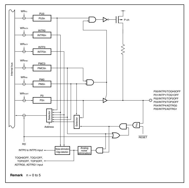
Figure 4-3. Block Diagram of P00 to P05 Pins
