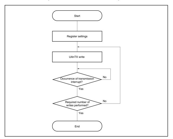
Figure 12-4. Continuous Transmission Processing Flow
