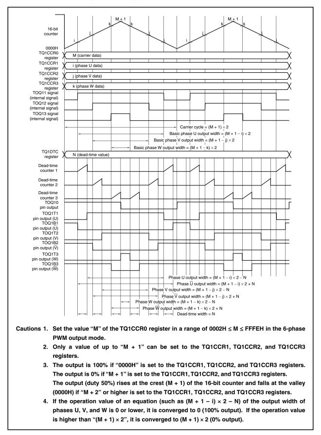
Figure 9-6. Timing Chart of 6-Phase PWM Output Mode
