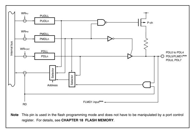
Figure 4-21. Block Diagram of PDL0 to PDL7 Pins
