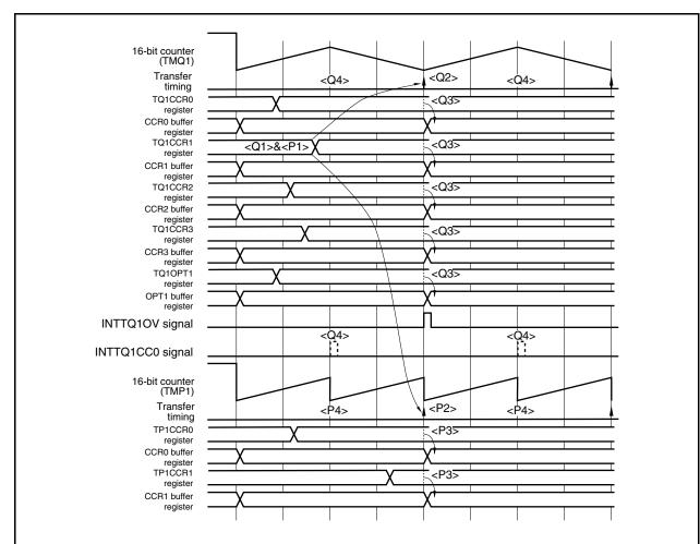
Figure 9-31. Basic Operation in Intermittent Batch Rewrite Mode
