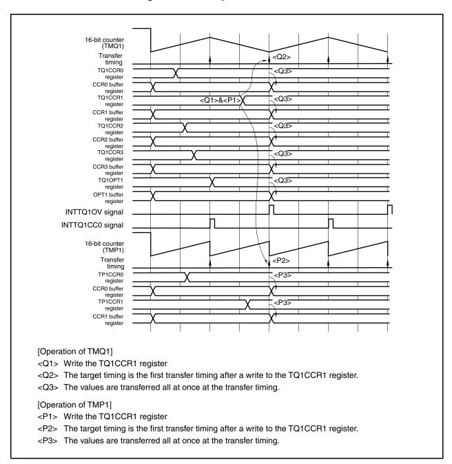
Figure 9-26. Basic Operation in Batch Mode
