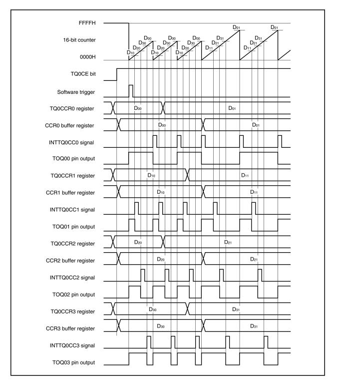
In order to transfer data from the TQ0CCRa register to the CCRa buffer register, the TQ0CCR1 register must be written.
