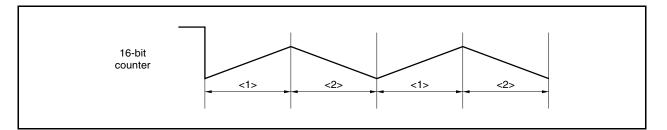
The transfer timing in Figure 9-28 is at the point where the crest timing occurs. While the 16-bit counter is counting down, the cycle changes and an asymmetrical triangular wave is output. Because the cycle changes, rewrite the duty factor (voltage data value).
