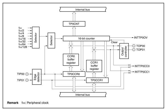
Figure 6-2. TMP1 Block Diagram
