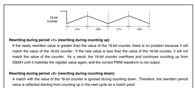
Figure 9-22. Example of Rewriting TQ1CCR0 Register
