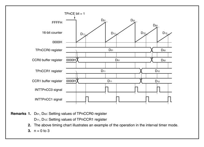
Figure 6-6. Timing of Anytime Write
