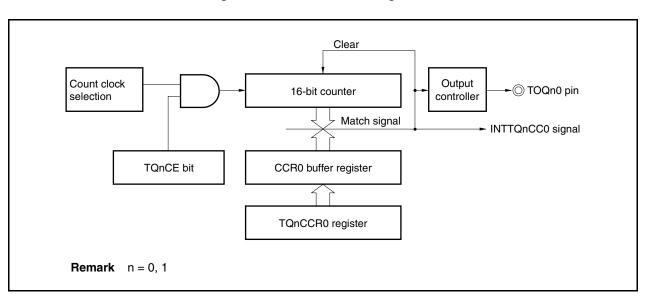
Figure 7-8. Interval Timer Configuration
