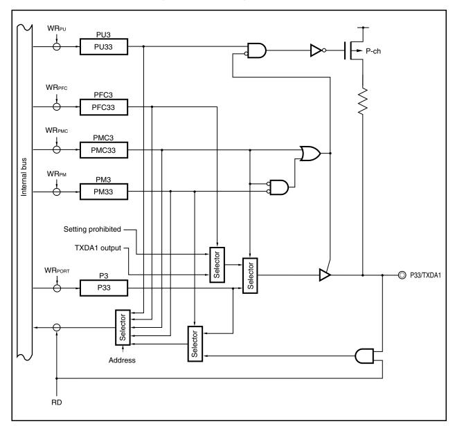
Figure 4-16. Block Diagram of P33 Pin
