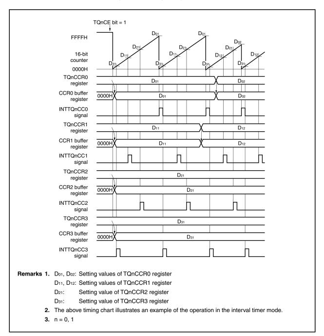
Figure 7-5. Timing of Anytime Write
