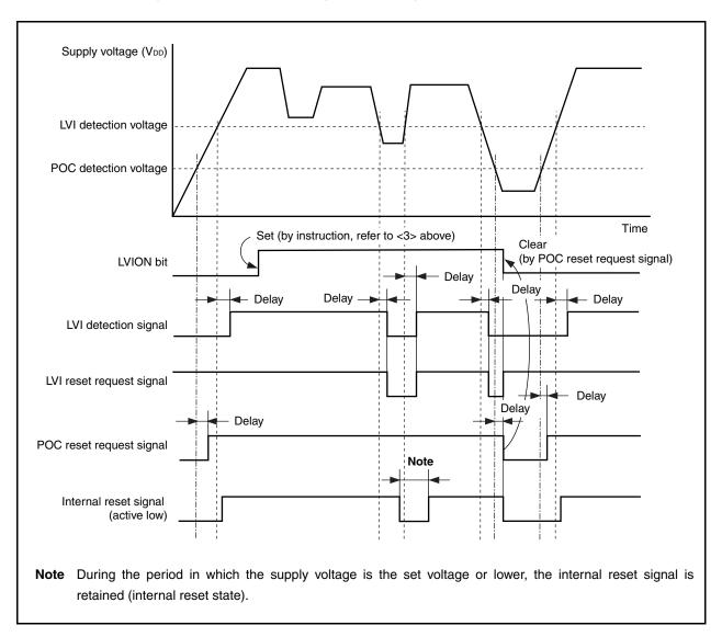
Figure 16-5. Operation Timing of Low-Voltage Detector (LVIMD Bit = 1)
