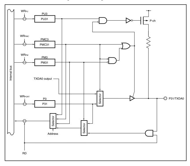
Figure 4-14. Block Diagram of P31 Pin
