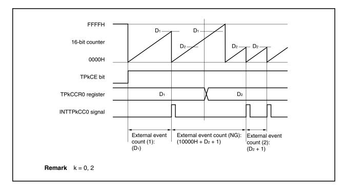
If the value of the TPkCCR0 register is changed from  $D_1$  to  $D_2$  while the count value is greater than  $D_2$  but less than  $D_1$ , the count value is transferred to the CCR0 buffer register as soon as the TPkCCR0 register has been rewritten. Consequently, the value that is compared with the 16-bit counter is  $D_2$ .
