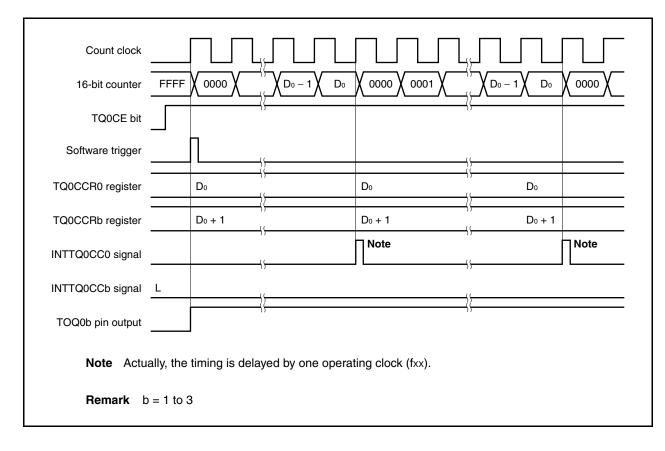
To output a 100% waveform, set a value of (set value of TQ0CCR0 register + 1) to the TQ0CCRb register. If the set value of the TQ0CCR0 register is FFFFH, 100% output cannot be produced.
