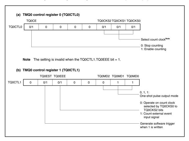
Figure 7-28. Register Setting in One-Shot Pulse Output Mode (1/3)
