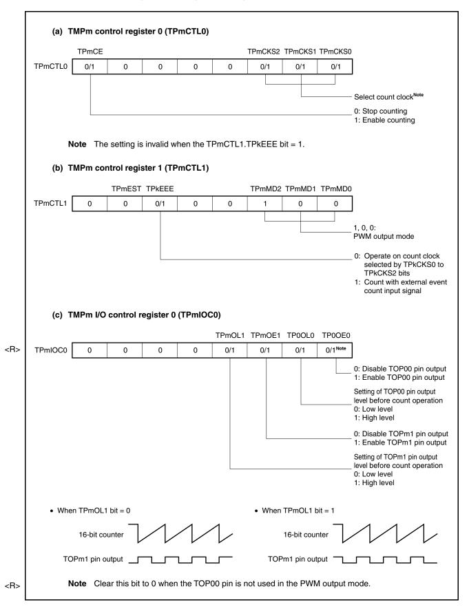
Figure 6-33. Register Setting in PWM Output Mode (1/2)
