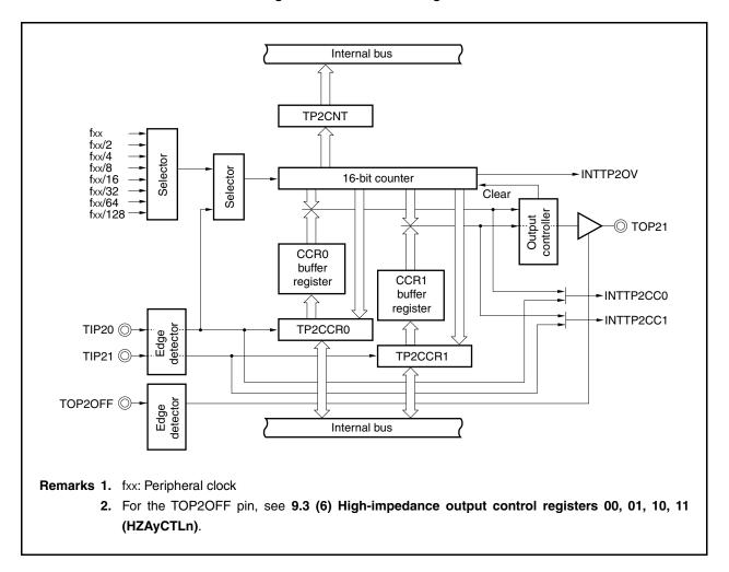
Figure 6-3. TMP2 Block Diagram
