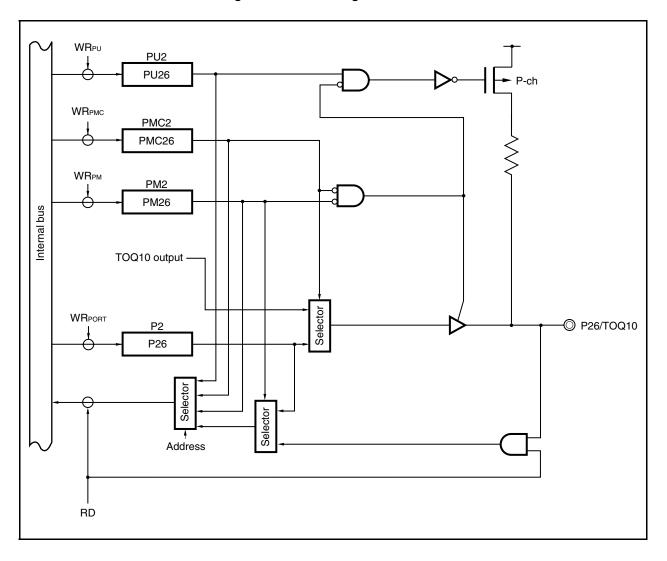
Figure 4-12. Block Diagram of P26 Pin
