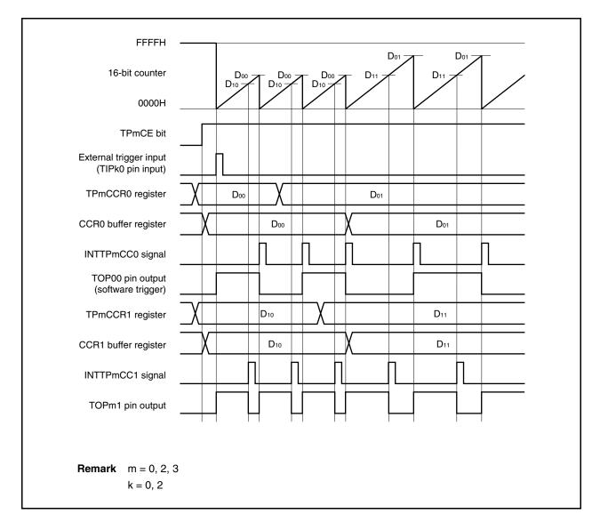
In order to transfer data from the TPmCCRa register to the CCRa buffer register, the TPmCCR1 register must be written.
