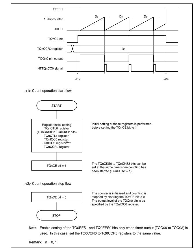
Figure 7-11. Software Processing Flow in Interval Timer Mode
