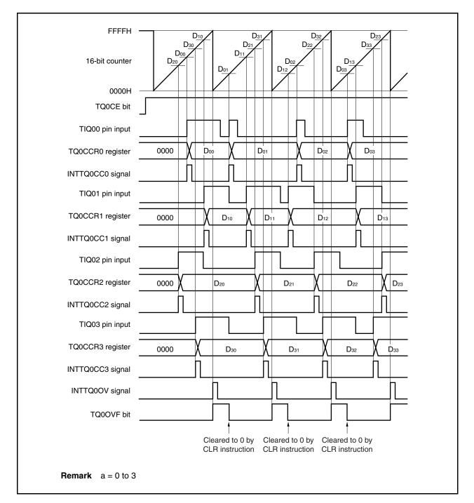
Figure 7-36. Basic Timing in Free-Running Timer Mode (Capture Function)
