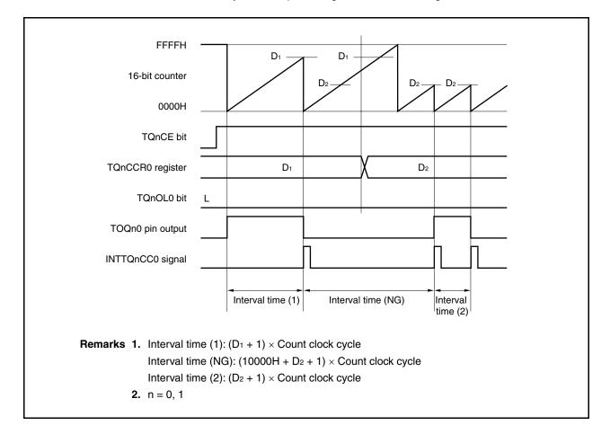
If the value of the TQnCCR0 register is changed from  $D_1$  to  $D_2$  while the count value is greater than  $D_2$  but less than  $D_1$ , the count value is transferred to the CCR0 buffer register as soon as the TQnCCR0 register has been rewritten. Consequently, the value of the 16-bit counter that is compared is  $D_2$ .
