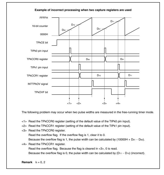
When two capture registers are used, and if the overflow flag is cleared to 0 by one capture register, the other capture register may not obtain the correct pulse width.
