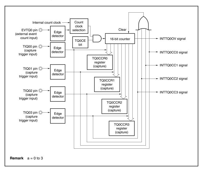
Figure 7-40. Configuration in Pulse Width Measurement Mode
