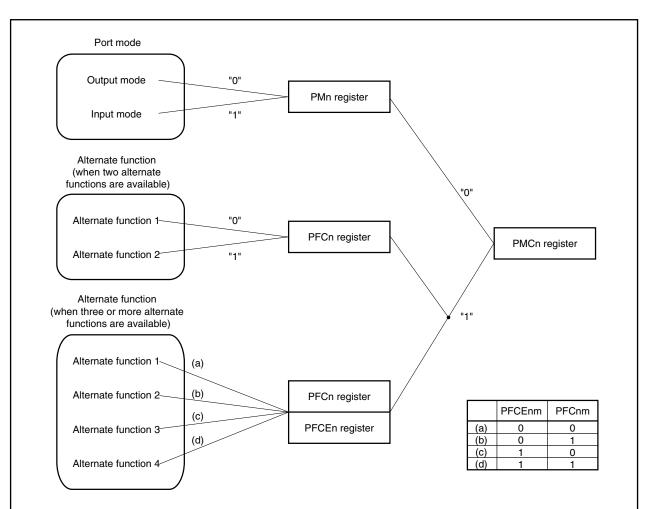
Figure 4-2. Register Settings and Pin Functions
