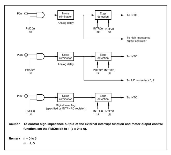
A noise elimination function is included as an alternate function of port 0.
