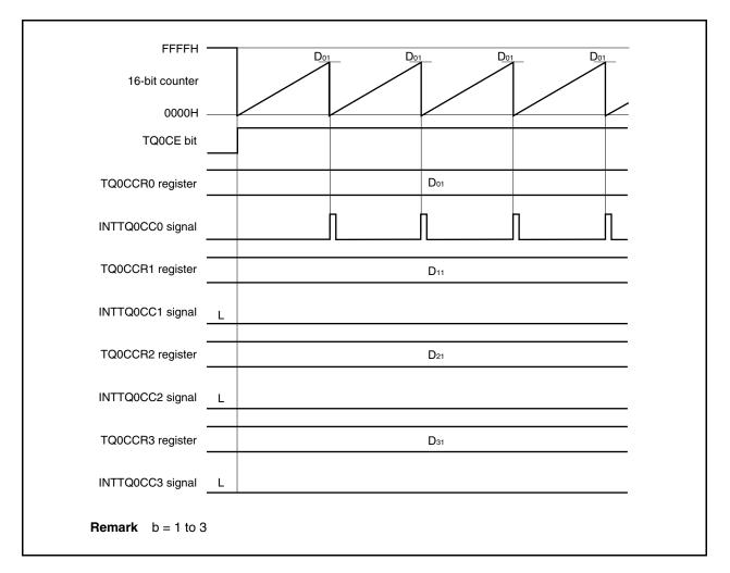
Figure 7-21. Timing Chart When Do1 < Db1
