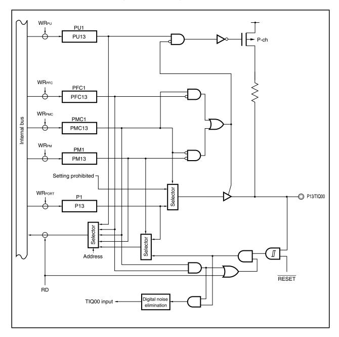
Figure 4-7. Block Diagram of P13 Pin
