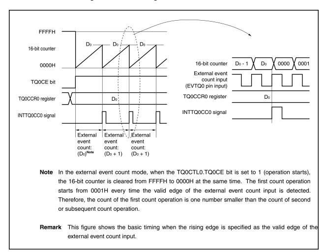
Figure 7-16. Basic Timing in External Event Count Mode
