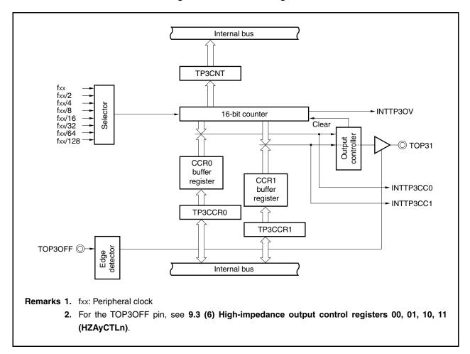
Figure 6-4. TMP3 Block Diagram
