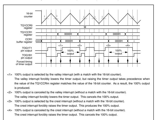
Figure 9-10. 100% PWM Output Waveform (with Dead Time)
