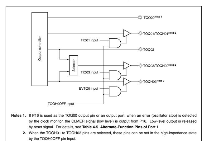
Figure 7-2. TMQ0 Output Pin Configuration
