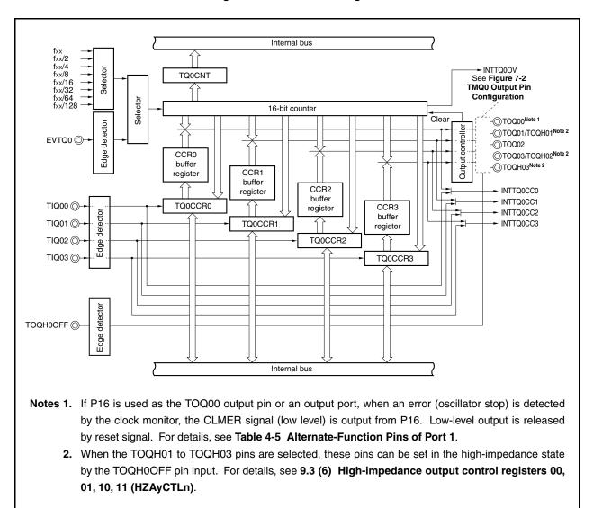
Figure 7-1. TMQ0 Block Diagram
