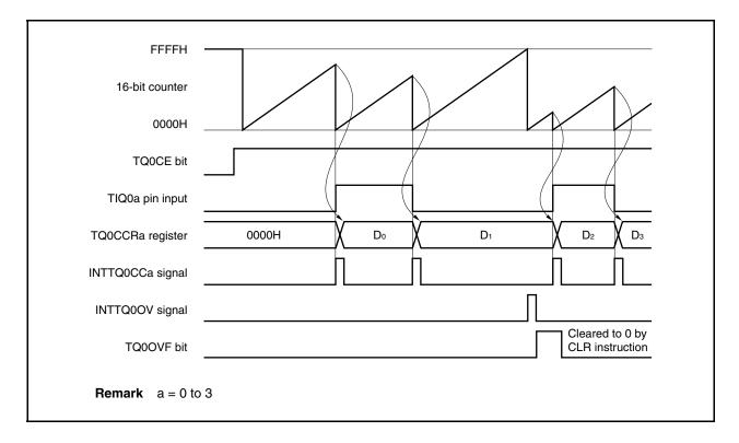
Figure 7-41. Basic Timing in Pulse Width Measurement Mode
