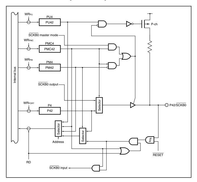
Figure 4-19. Block Diagram of P42 Pin
