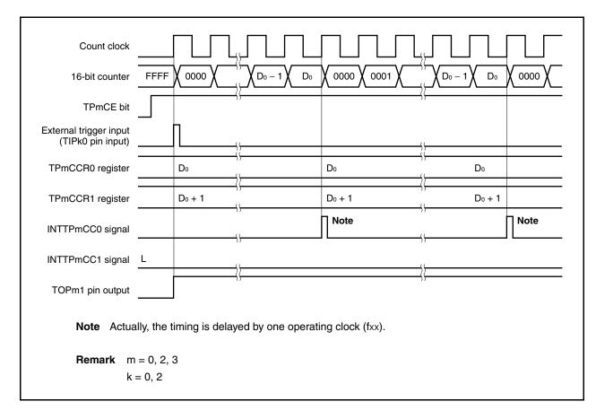
To output a 100% waveform, set a value of (set value of TPmCCR0 register + 1) to the TPmCCR1 register. If the set value of the TPmCCR0 register is FFFFH, 100% output cannot be produced.
