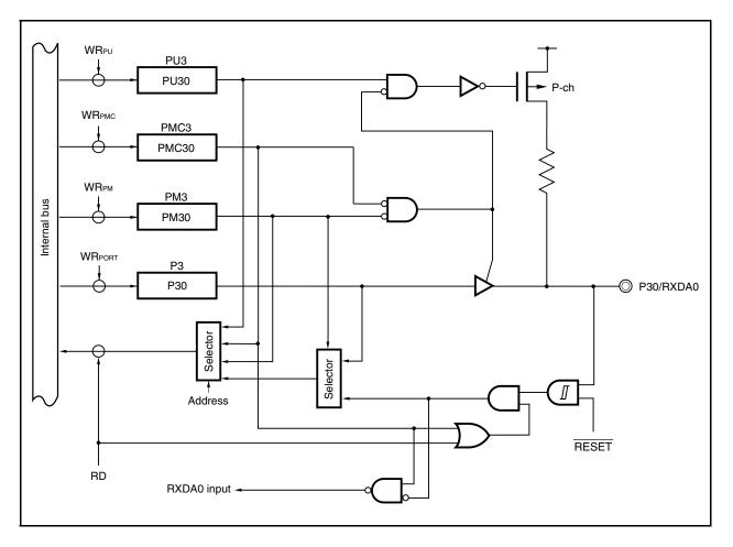
Figure 4-13. Block Diagram of P30 Pin
