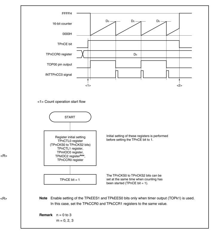
Figure 6-12. Software Processing Flow in Interval Timer Mode (1/2)
