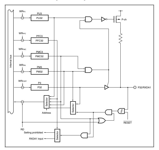
Figure 4-15. Block Diagram of P32 Pin
