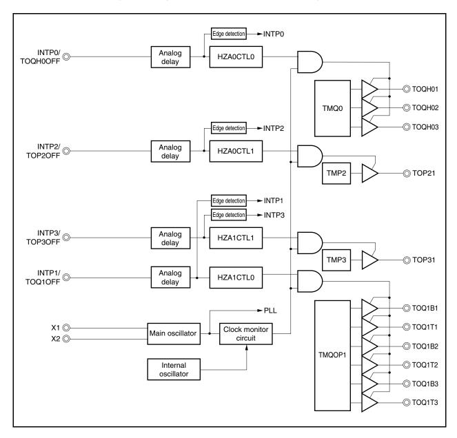
Figure 9-4. High-Impedance Output Controller Configuration
