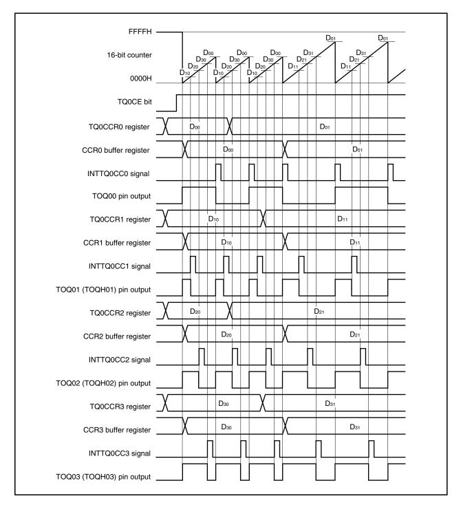
To transfer data from the TQ0CCRa register to the CCRa buffer register, the TQ0CCR1 register must be written.
