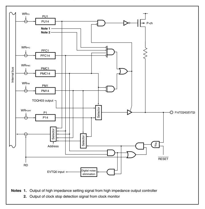
Figure 4-8. Block Diagram of P14 Pin
