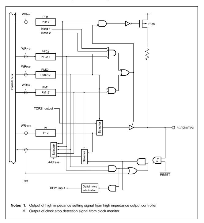
Figure 4-10. Block Diagram of P17 Pin
