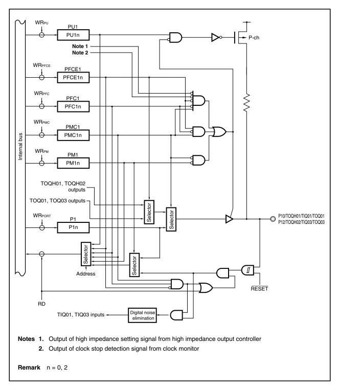
Figure 4-5. Block Diagram of P10 and P12 Pins
