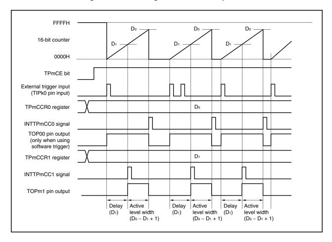
Figure 6-28. Basic Timing in One-Shot Pulse Output Mode
