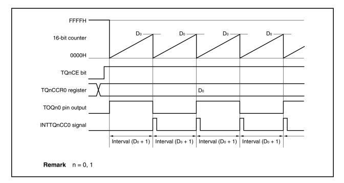
When the TQnCE bit is set to 1, the value of the 16-bit counter is cleared from FFFFH to 0000H in synchronization with the count clock, and the counter starts counting. At this time, the output of the TOQn0 pin is inverted. Additionally, the set value of the TQnCCR0 register is transferred to the CCR0 buffer register.
