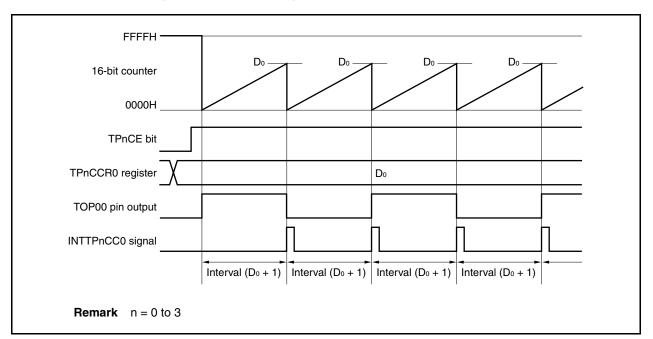
When the TPnCE bit is set to 1, the value of the 16-bit counter is cleared from FFFFH to 0000H in synchronization with the count clock, and the counter starts counting. At this time, the output of the TOP00 pin is inverted. Additionally, the set value of the TPnCCR0 register is transferred to the CCR0 buffer register.
