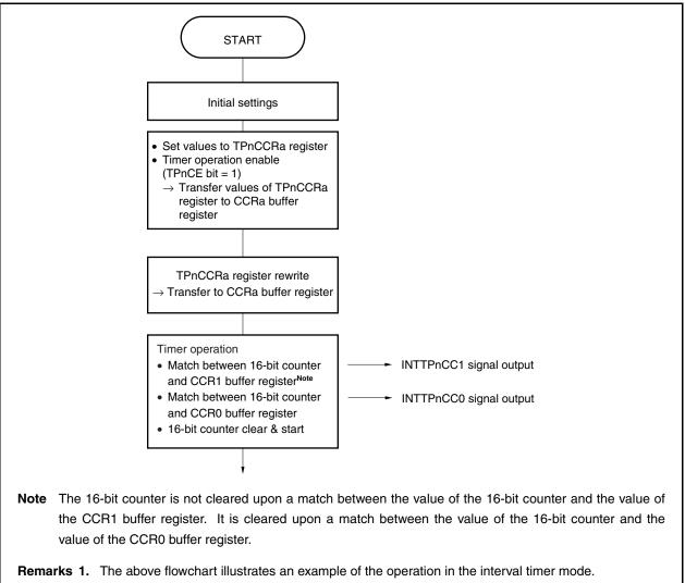
Figure 6-5. Flowchart of Basic Operation for Anytime Write
