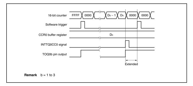
If the trigger is detected immediately before the INTTQ0CC0 signal is generated, the INTTQ0CC0 signal is not generated. The 16-bit counter is cleared to 0000H, the TOQ0b pin is asserted, and the counter continues counting. Consequently, the inactive period of the PWM waveform is shortened.
