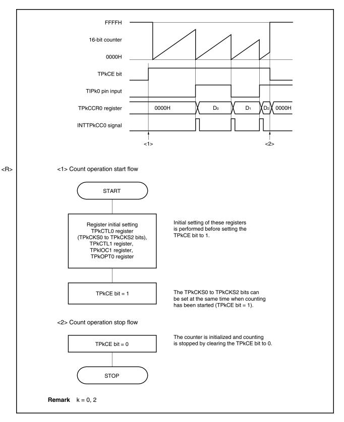
Figure 6-44. Software Processing Flow in Pulse Width Measurement Mode
