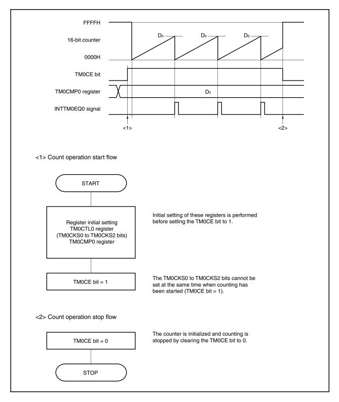
Figure 8-5. Software Processing Flow in Interval Timer Mode
