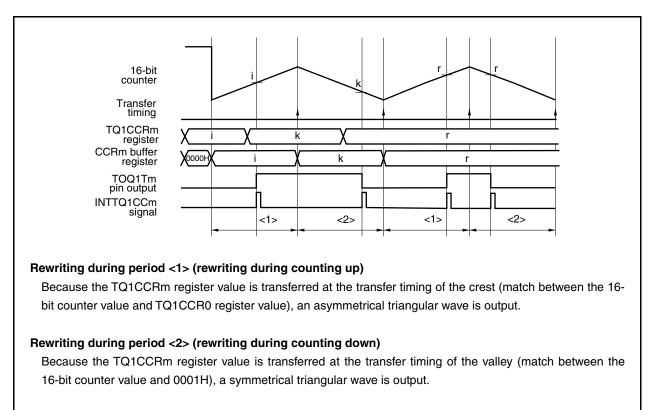
Figure 9-30. Example of Rewriting TQ1CCRm Register
