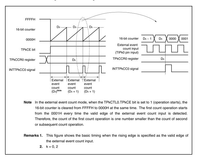
Figure 6-17. Basic Timing in External Event Count Mode
