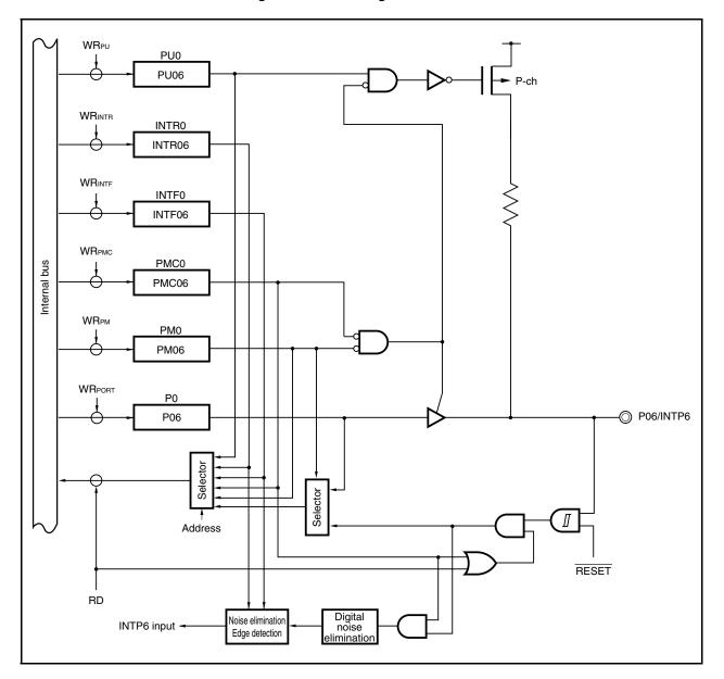
Figure 4-4. Block Diagram of P06 Pin
