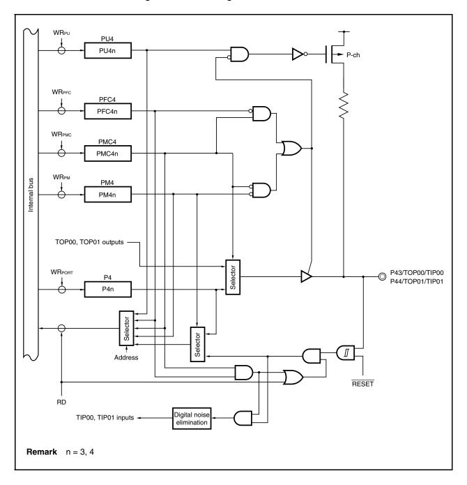
Figure 4-20. Block Diagram of P43 and P44 Pins
