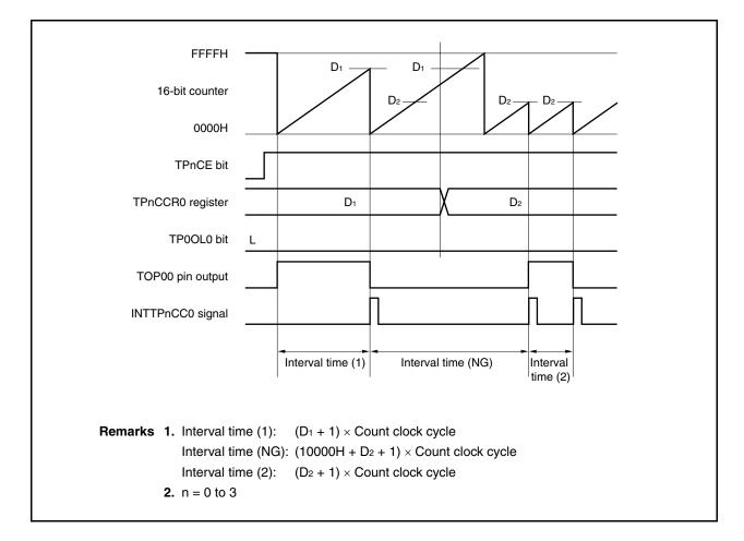
If the value of the TPnCCR0 register is changed from  $D_1$  to  $D_2$  while the count value is greater than  $D_2$  but less than  $D_1$ , the count value is transferred to the CCR0 buffer register as soon as the TPnCCR0 register has been rewritten. Consequently, the value of the 16-bit counter that is compared is  $D_2$ .
