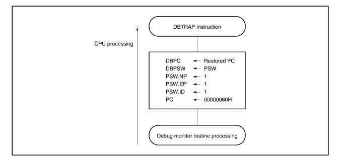
Figure 14-11. Debug Trap Processing
