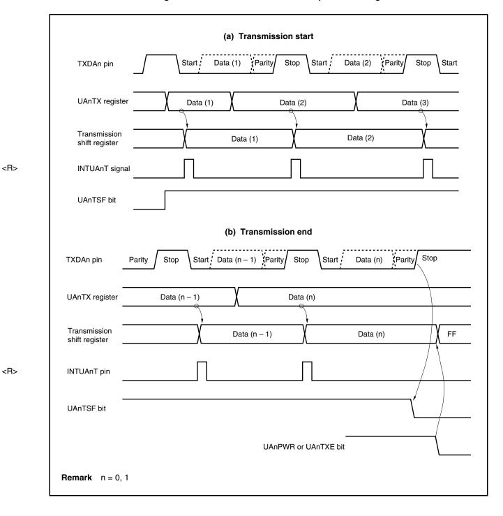
Figure 12-5. Continuous Transmission Operation Timing
