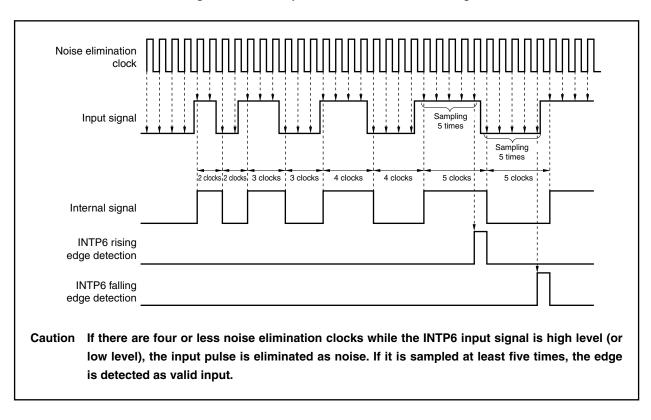
Figure 4-22. Example of Noise Elimination Timing
