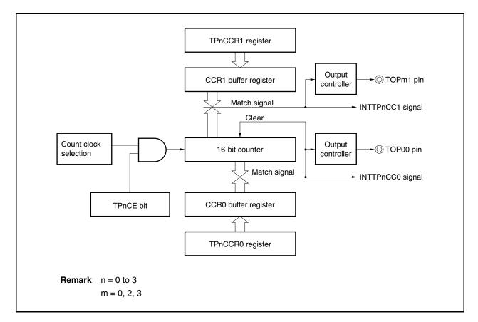
When the TPnCCR1 register is set to the same value as the TPnCCR0 register, the INTTPnCC1 signal is generated at the same timing as the INTTPnCC0 signal and the TOPm1 pin output is inverted. In other words, a PWM waveform with a duty factor of 50% can be output from the TOPm1 pin.
