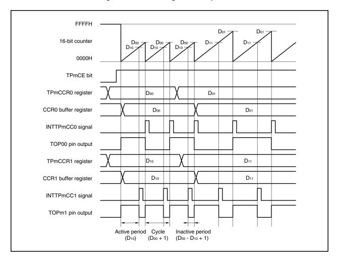
Figure 6-32. Basic Timing in PWM Output Mode
