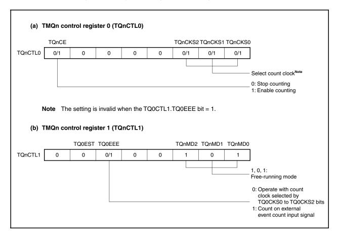
Figure 7-37. Register Setting in Free-Running Timer Mode (1/3)
