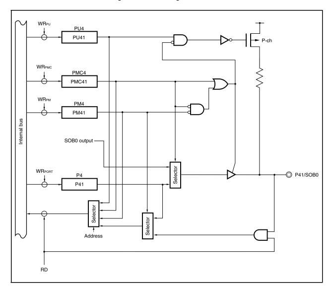
Figure 4-18. Block Diagram of P41 Pin
