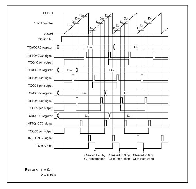
Figure 7-35. Basic Timing in Free-Running Timer Mode (Compare Function)
