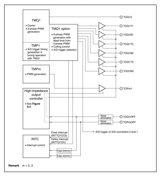
Figure 9-1. Block Diagram of Motor Control
