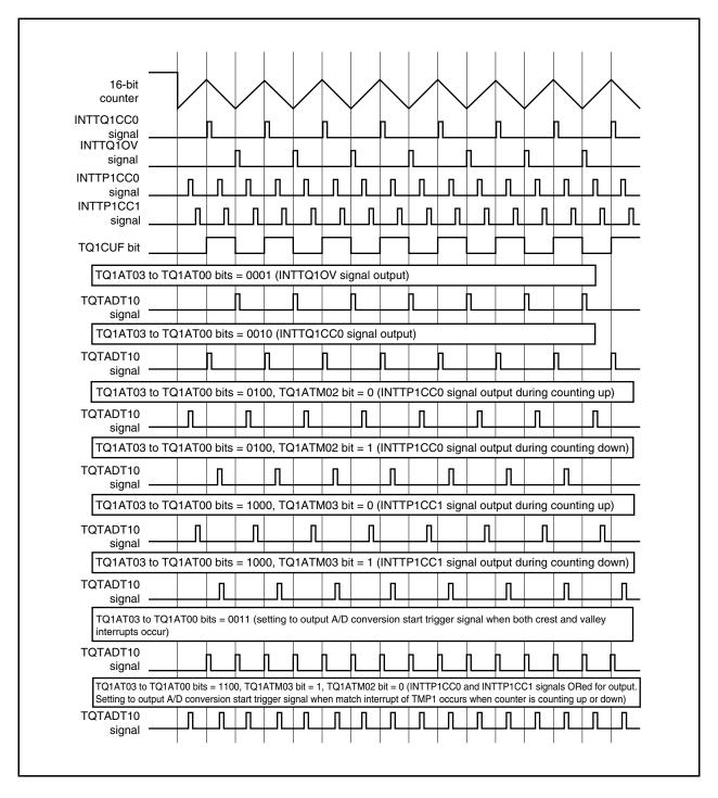
Figure 9-38. Example of A/D Conversion Start Trigger (TQTADT10) Signal Output (TQ1OPT1.TQ1ICE Bit = 1, TQ1OPT1.TQ1IDE Bit = 1, TQ1OPT1.TQ1ID4 to TQ1OPT1.TQ1ID0 Bits = 00000: Without Interrupt Culling)
