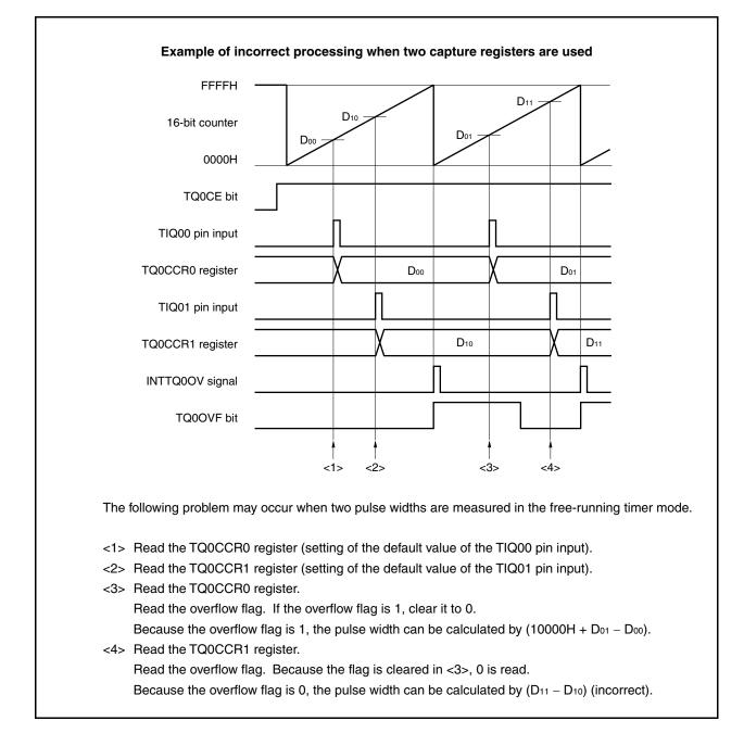
When two capture registers are used, and if the overflow flag is cleared to 0 by one capture register, the other capture register may not obtain the correct pulse width.
