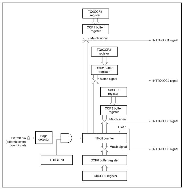
Figure 7-19. Configuration of TQ0CCR1 to TQ0CCR3 Registers
