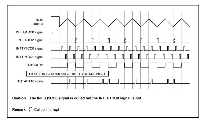
(1) Operation under boundary condition (operation when 16-bit counter matches INTTP1CC0 signal)
