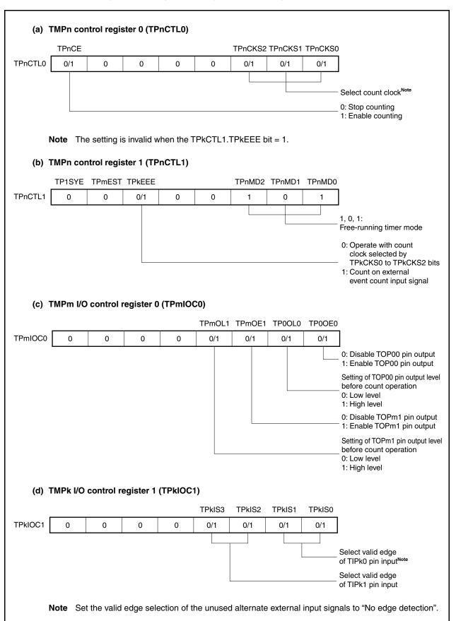
Figure 6-38. Register Setting in Free-Running Timer Mode (1/2)
