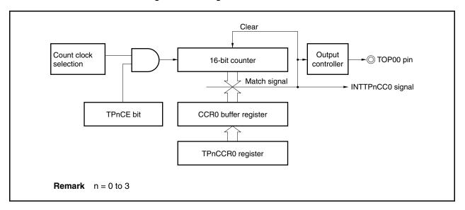
Figure 6-9. Configuration of Interval Timer
