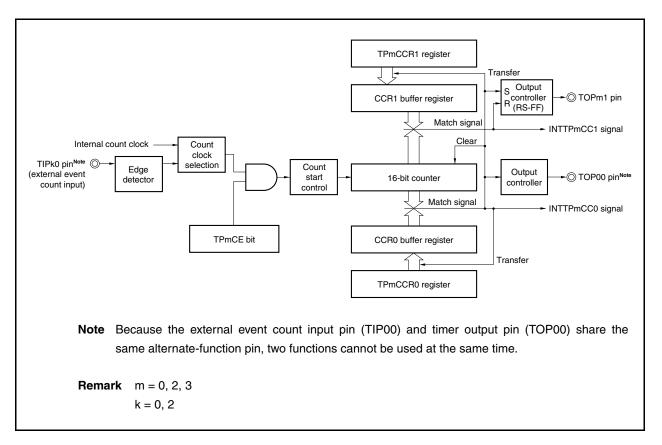
Figure 6-31. Configuration in PWM Output Mode
