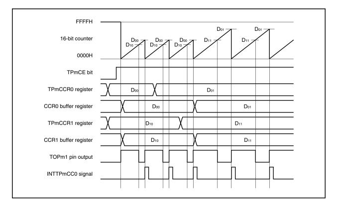
To transfer data from the TPmCCRa register to the CCRa buffer register, the TPmCCR1 register must be written.
