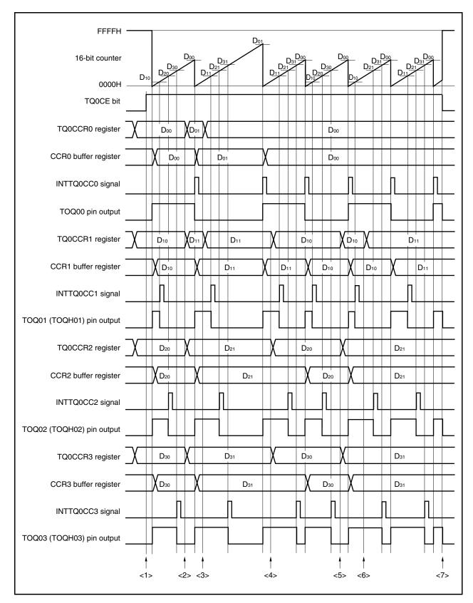
Figure 7-33. Software Processing Flow in PWM Output Mode (1/2)
