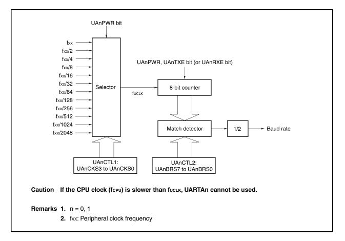
Figure 12-9. Configuration of Baud Rate Generator
