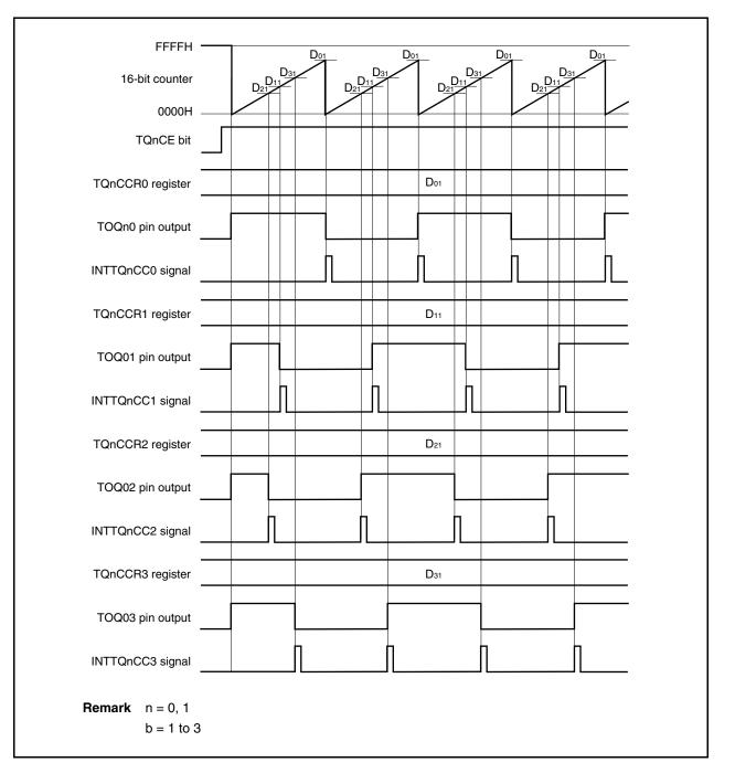
Figure 7-13. Timing Chart When Do1 ≥ Db1
