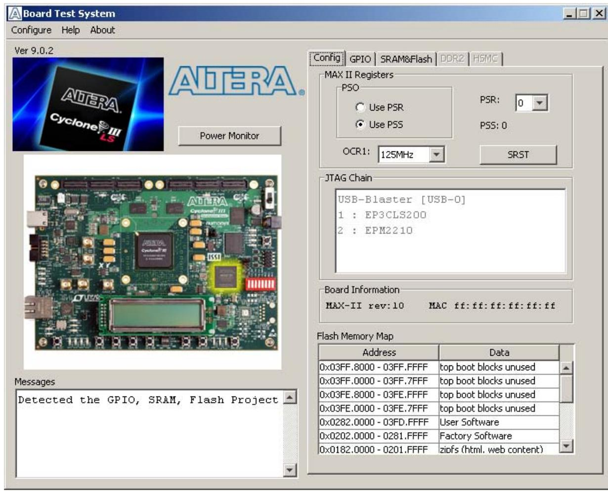
Several designs are provided to test the major board features. Each design provides data for one or more tabs in the application. The Configure menu identifies the appropriate design to download to the FPGA for each tab.
