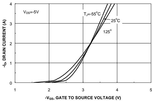
**Figure 5. Transfer Characteristics.**
