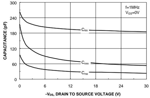
**Figure 8. Capacitance Characteristics.**
