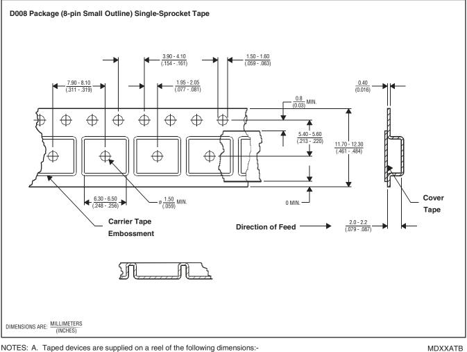
330 +0.0/-4.0 Reel diameter: (12.992 +0.0/-.157)  $100 \pm 2.0$ Reel hub diameter: (3.937 ± .079) 13.0 ± 0.2 (.512 ± .008) Reel axial hole:
