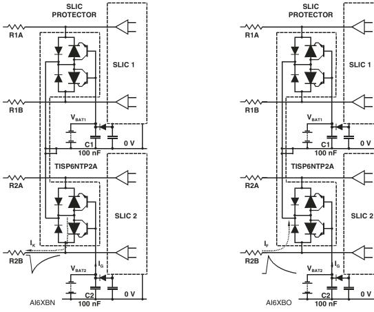
Figure 2. Negative Overvoltage Condition
