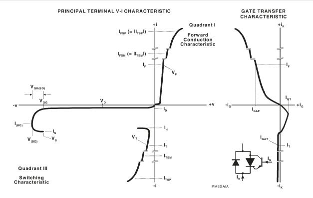
Figure 1. Principal Terminal And Gate Transfer Characteristics
