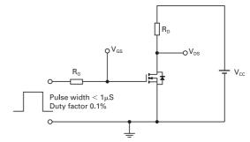
Switching time test circuit
