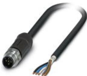
Sensor/Actuator cable, 5-position, PE-X/PE-X halogen-free, black-gray RAL 7021, shielded, Plug straight M12, A-coded, on free cable end, Cable length: 10 m, for outdoor applications, with high-grade steel knurl
