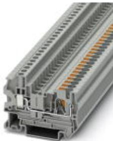
Feed-through terminal block, connection method: Push-in connection, Screw connection, cross section: 0.2 mm<sup>2</sup> - 6 mm<sup>2</sup>, AWG: 24 - 12, width: 6.2 mm, color: white, mounting: NS 35/7,5, NS 35/15
