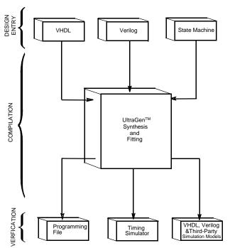
Figure 1. Warp VHDL Design Flow
