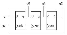
Figure 3. Three-Bit Shift Register Circuit Design
