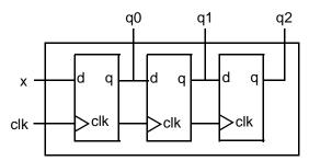
Figure 5. Three-Bit Shift Register Circuit Design
