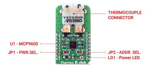
There are four ALERT lines present on the MCP9600. Those lines can be programmed by the I2C to be set to a HIGH logic level when certain temperature thresholds are reached. The lines are routed to the AN, RST, PWM and INT pins of the mikroBUS<sup>TM</sup>.
