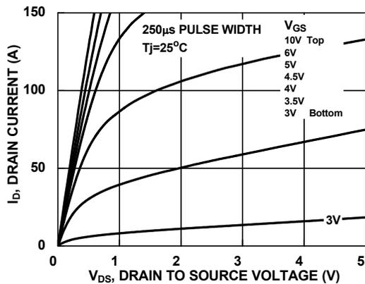
Figure 9. Saturation Characteristics
