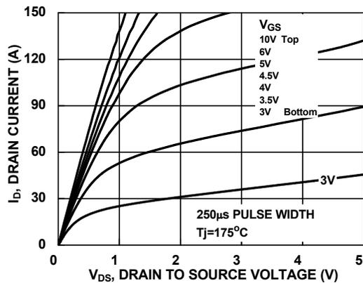
Figure 10. Saturation Characteristics
