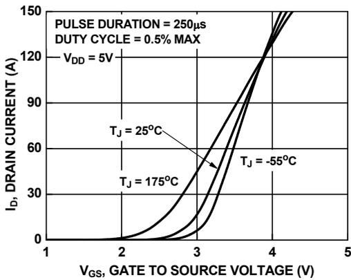
Figure 7. Transfer Characteristics
