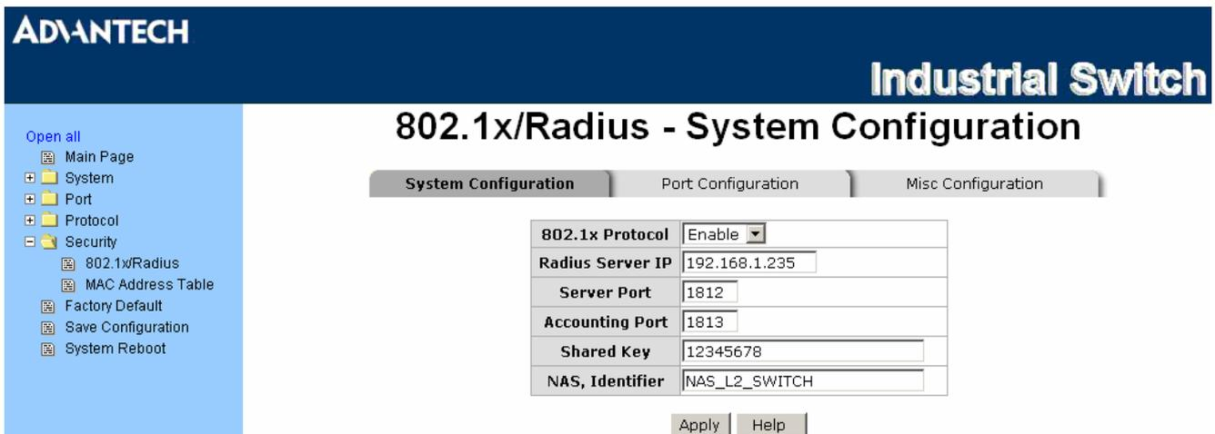
Figure 3.3-44 802.1x/Radius System Configuration
