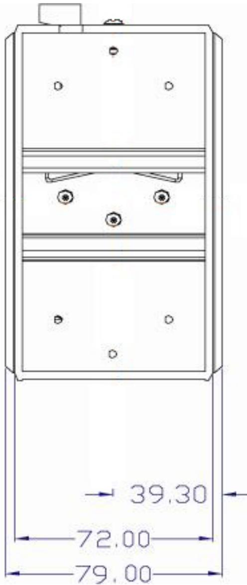
Figure 2.2-3 Rear View of EKI-7559MI/SI
