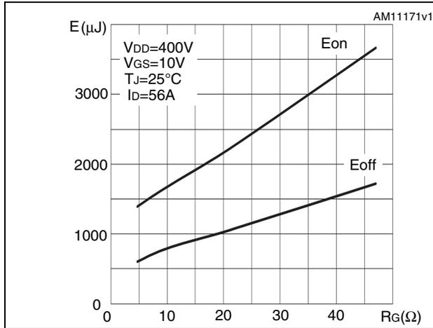
1.  $E_{on}$  including reverse recovery of a SiC diode.
