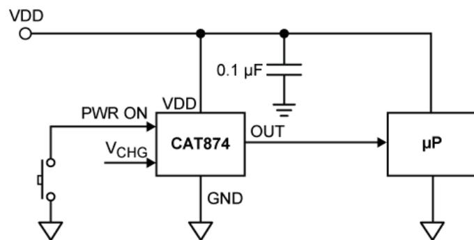
Figure 1. Application Schematic
