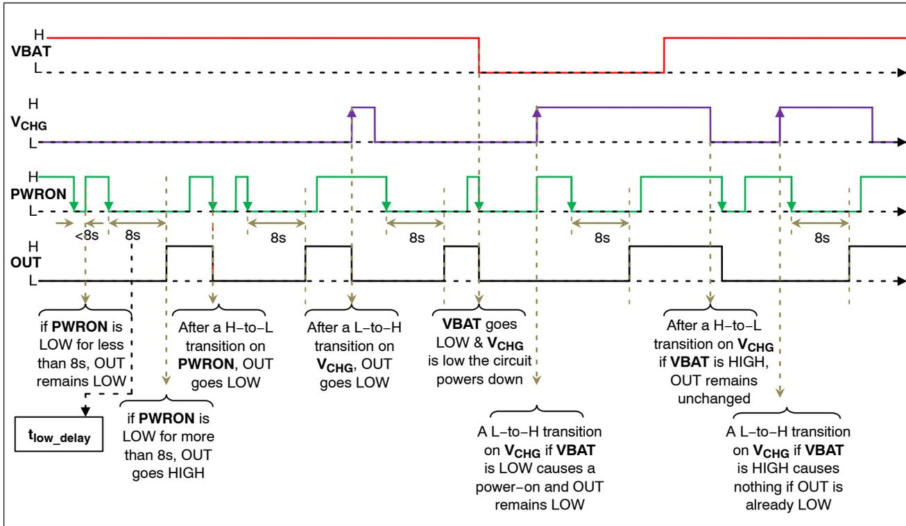
Figure 3. Timing Waveforms
