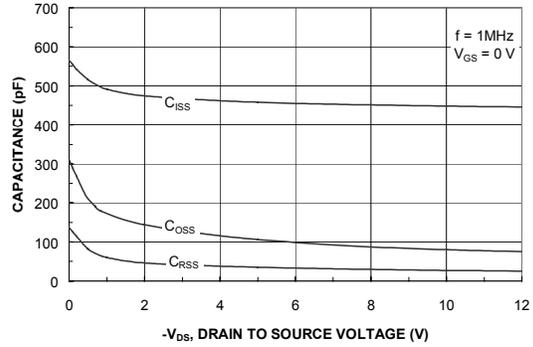
Figure 8. Capacitance Characteristics.
