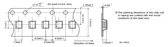
Dimension of the Cavity is measured at the bottom side.
